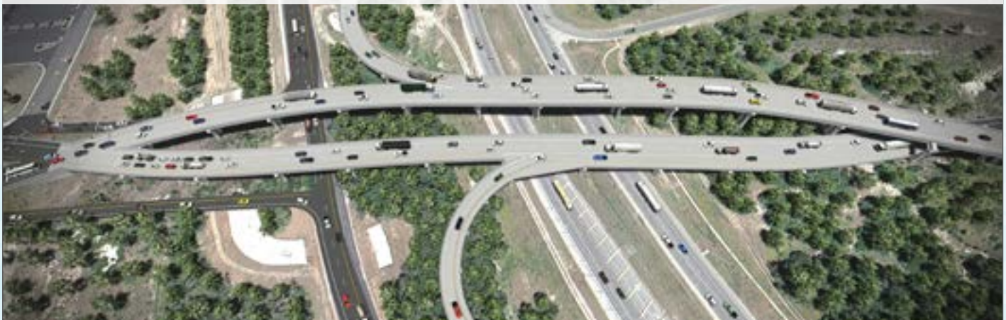
The Zachry Team’s proposed modified diverging diamond interchange for the Loop 1604 and SH 151 interchange
