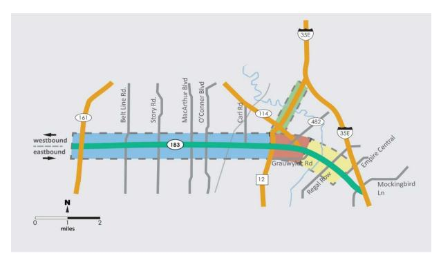
**Project Limits:** The SH 183 Managed Lane Project limits are generally described as: from just west of SH 161 to just west of IH 35E, and on Loop 12 from SH 183 to just south of IH 35E.
