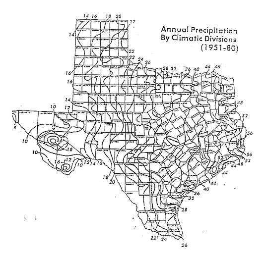
Figure 1. Rainfall graph for determining regional soil testing requirements
