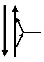
An interchange which provides access to only one side of the mainlanes. No overpass of the mainlanes is provided.
