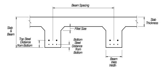
Figure 4. T-Beam Diagram.
