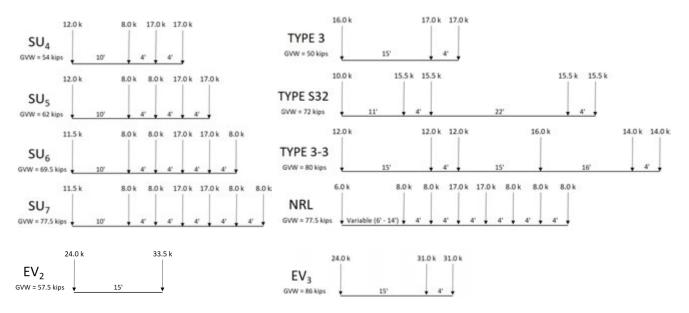
Figure 14. SHV, AASHTO Type 3, NRL and EV Load Configurations
