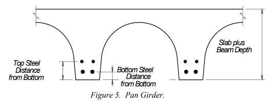
[Total Area of Steel], in square inches, refers to the reinforcing steel running longitudinally within the T-beam. The depth of this steel measured from the center of the bars in inches, is noted in the [Distance from Bottom] field. The spreadsheet allows for the input of two layers of steel. If the bridge being rated has more than two layers, the bottom layer area and distance should be entered in the fields for the bottom layer and the remaining reinforcement should be entered in the fields
