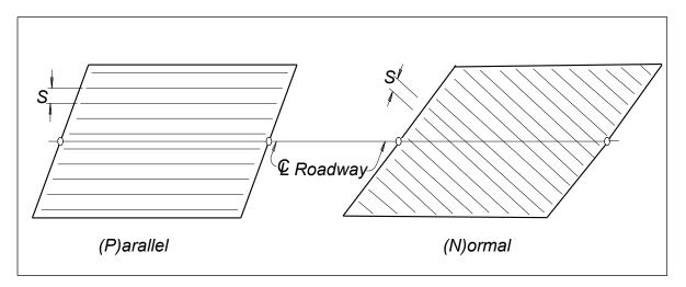
Figure 7. Flat Slab Steel Direction.
