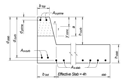
Figure 16. Curb for Flat Slab Bridges.
