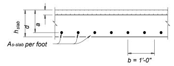
The depth of the stress block on the slab is as follows:
