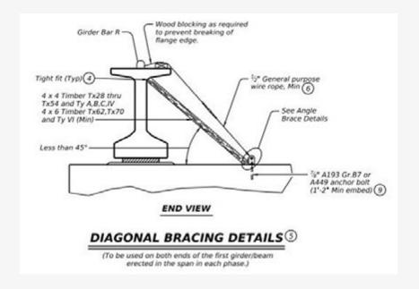
9 Anchor bolt may be drilled and epoxied in place. Provide 25k minimum pullout. Core drill hole.
