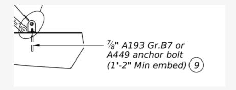
9) Anchor bolt may be drilled and epoxied in place. Provide 25k minimum pullout. Core drill hole.
