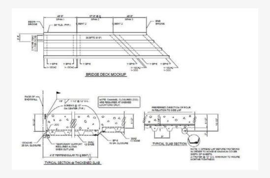
4.2.2. **Permanent Metal Decking.** Submit signed and sealed design calculations in addition to the required formwork drawings. Design and install formwork as shown on the plans and formwork drawings. The plans will govern in cases where the plans and the formwork drawings conflict.
