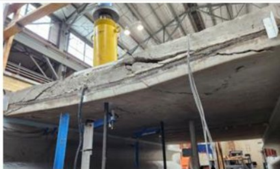
(b) Punching shear failure from bottom
