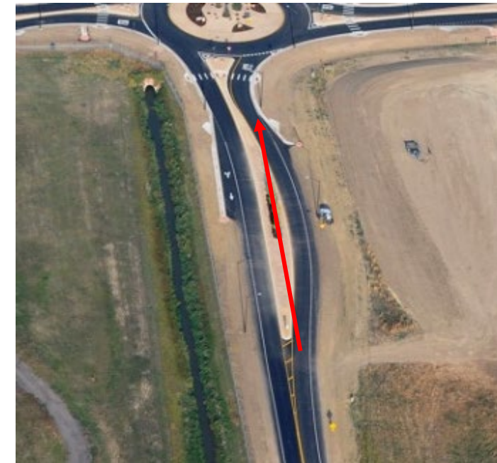
Above: The splitter island 'bump-out' is so wide that it deprives the driver of forward sight
