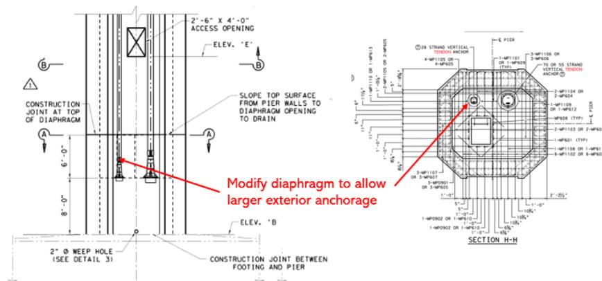
Figure 14 | Modifications will be required to the already built transition pier diaphragm
