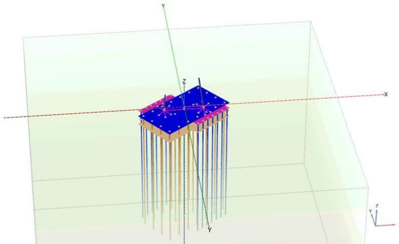
Figure 4 | Plaxis model of modified foundation (NT1)
