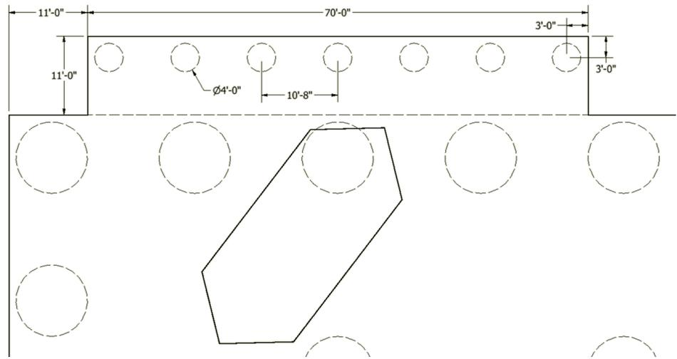
Figure 1 | Layout of additional drilled shafts
