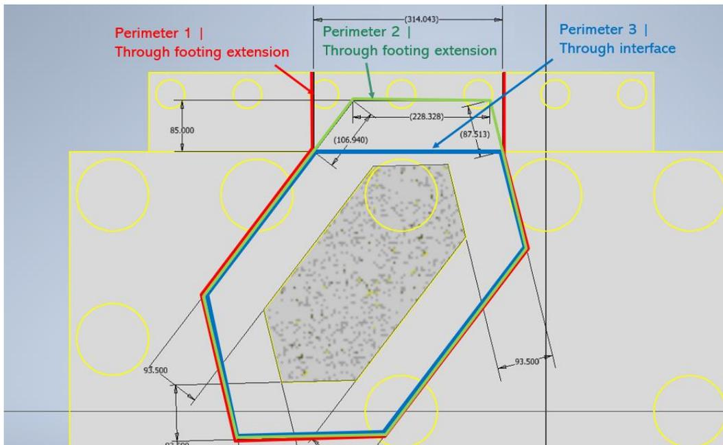
Figure 10 | Critical perimeters for two way action based on IBT Technical Memorandum
