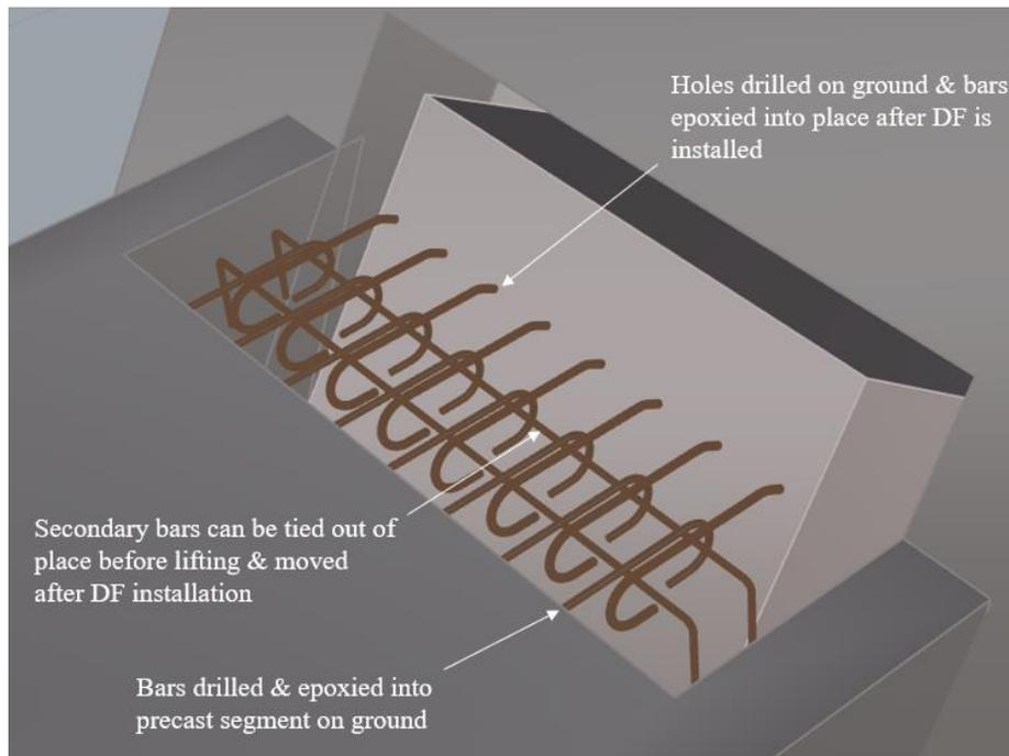
Figure 12. Proposed reinforcement installation sequence
