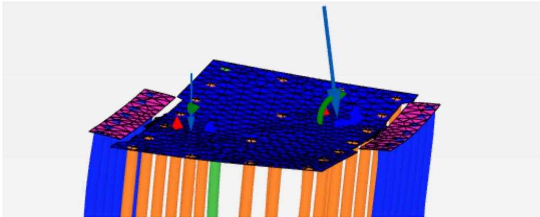
Figure 5: Deformed shape of the footing (1NT 270 deg. IBT input loads, OIF = 1.05)
