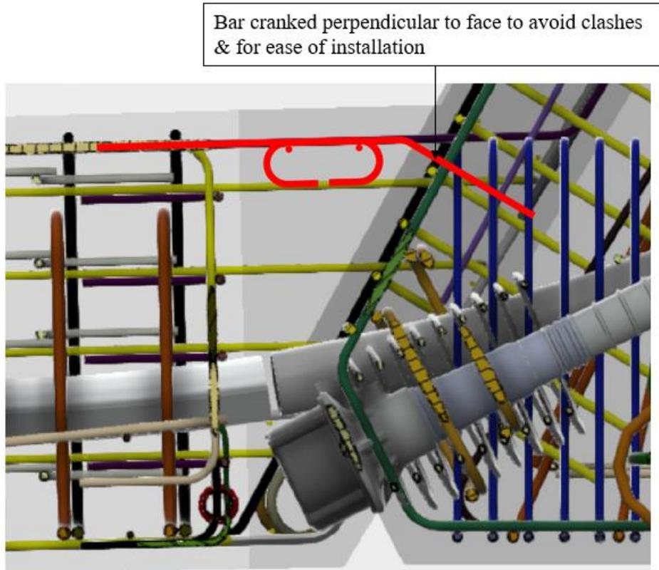
Figure 11. Proposed reinforcement layout. New reinforcement shown in red, all other reinforcement is existing.
