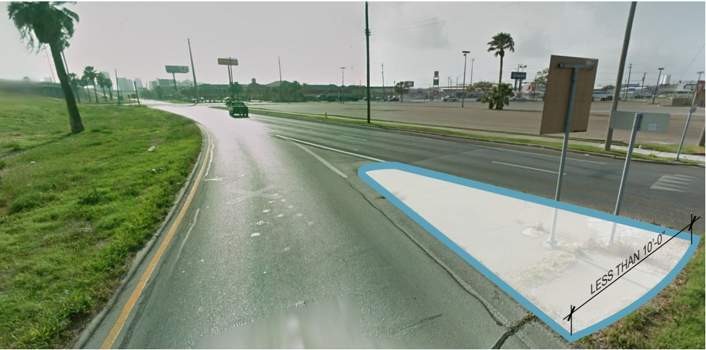
Figure 5.7 – Example delineating where enhanced riprap is not required
