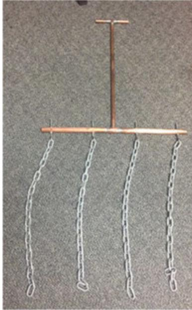
**Figure 2-2. A chain drag made from copper tubing and steel chain.**
