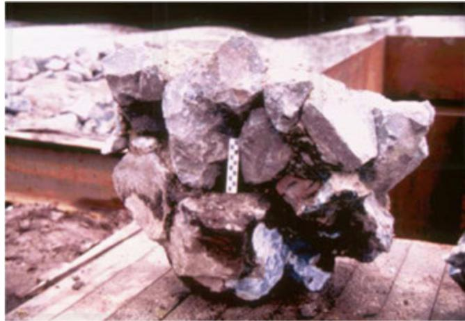
**Figure 13-3: Grouted Stone Protection – Conglomerates**
