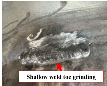
Weld toe after shallow grinding
