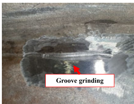
Crack removed prior to rewelding
