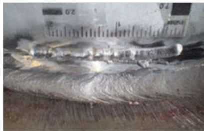
Grinding and grooving
