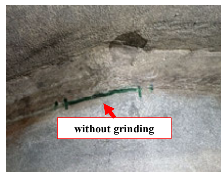
Crack left in place prior to rewelding
