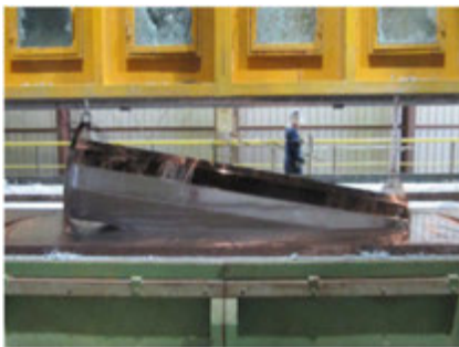
Thermal stress during galvanizing
