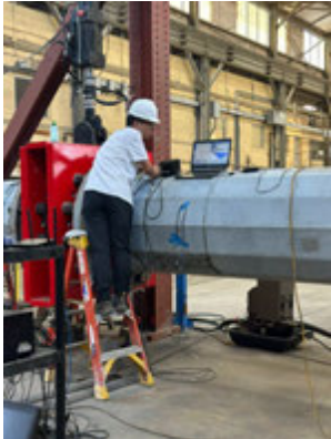
Crack monitoring (PAUT)
