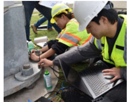
PAUT crack detection
