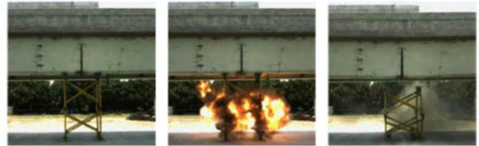
Figure 1.7: Second bridge fracture test
