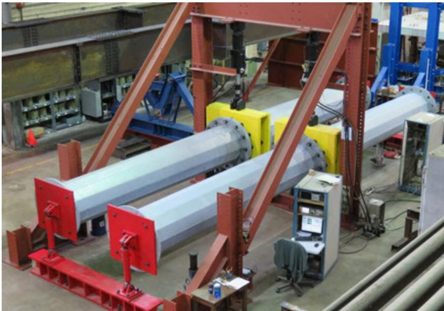
Tests at both UT and A&M on HMIP, COSS, and TSS Specimens. Cyclic loading to obtain cracks, study weld repair techniques and performance.
