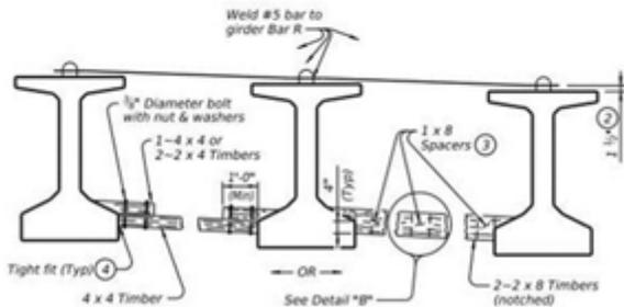
**FOR ERECTION BRACING, OPTION 2**
