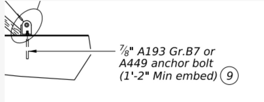
⑨ Anchor bolt may be drilled and epoxied in place. Provide 25k minimum pullout. Core drill hole.
