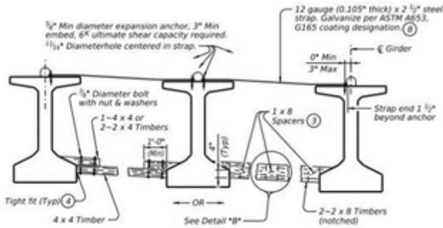
**FOR ERECTION BRACING, OPTION 1**
