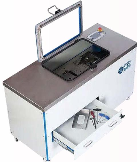
Overlay Cracking Test Setup
