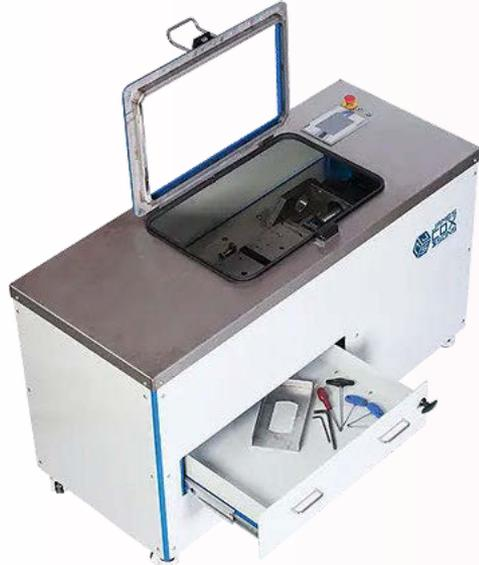
Overlay Cracking Test Setup
