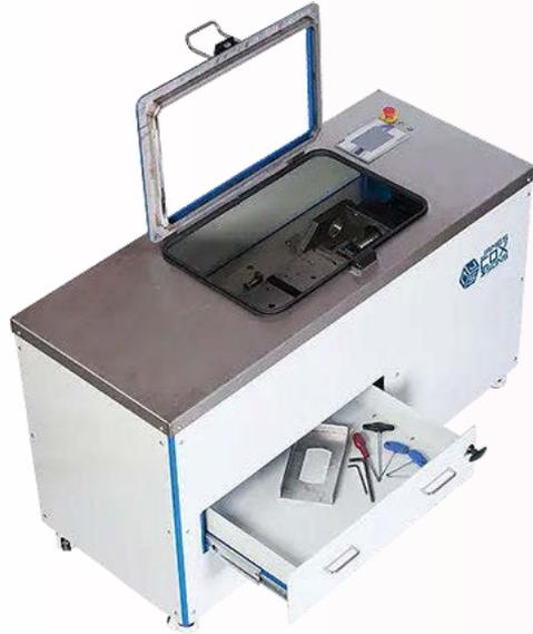
Overlay Cracking Test Setup
