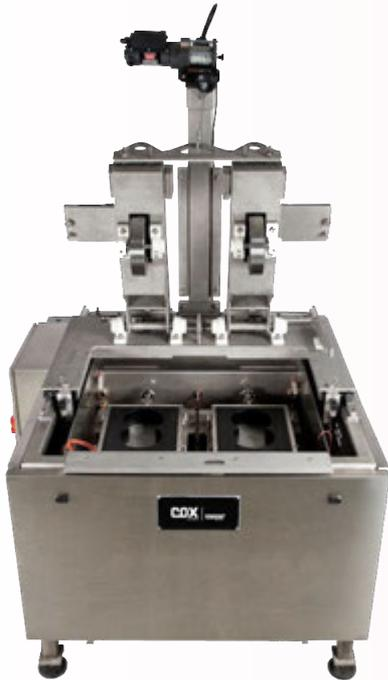
Hamburg Wheel-Tracking Test Setup
