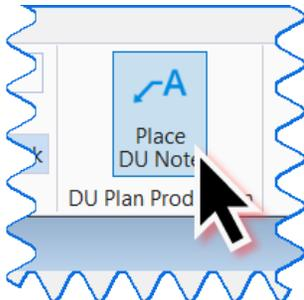
This will start the command to place a label/note in your drawing model. The “Place Note” toolbox should appear along with the Text Editor box.
