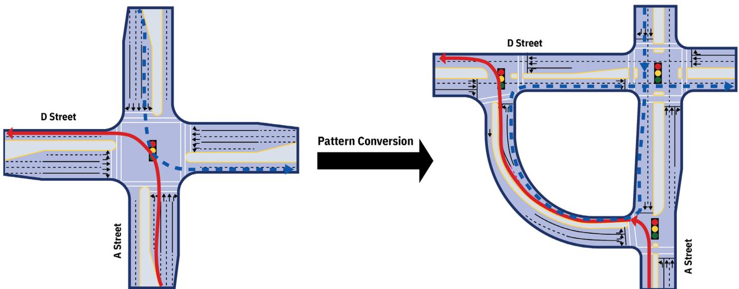
FIGURE 7 - TRADITIONAL INTERSECTION (LEFT) / QUADRANT ROADWAY (RIGHT) COMPARISON
