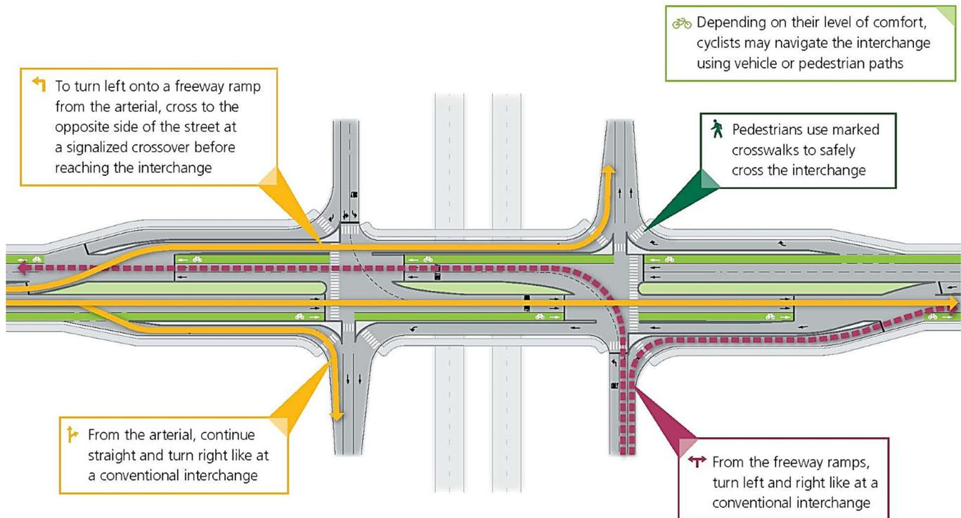
FIGURE 3 - DISPLACED LEFT TURN INTERCHANGE
