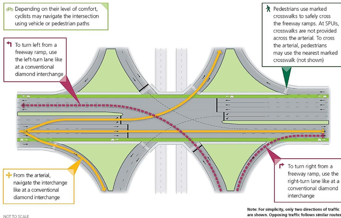
FIGURE 9 - SINGLE POINT URBAN INTERCHANGE (SPUI)
