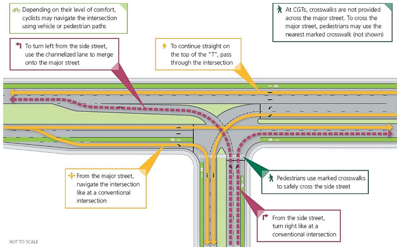
FIGURE 2 - CGT INTERSECTION (THREE-LEGGED DESIGN)
