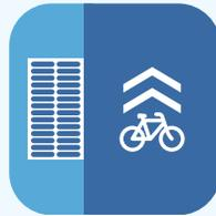
Locating **drainage grates** outside of the bikeway, to maximize the rideable space in the bikeway
