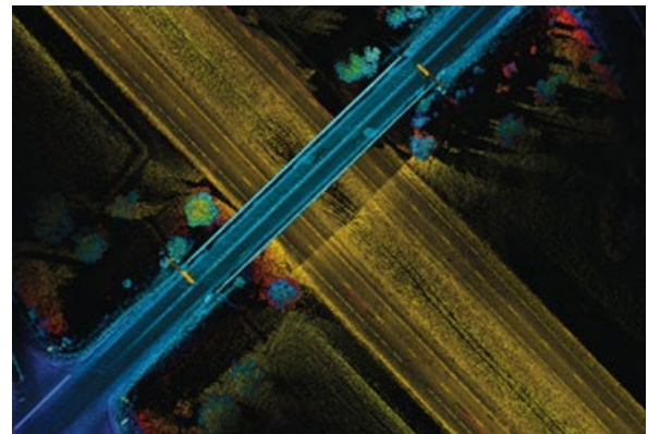
Figure 1: Mobile Lidar Point Cloud, colored by elevation
