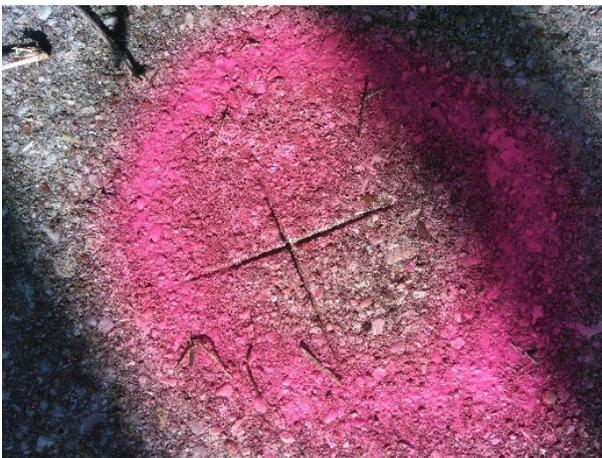
*Figure 1: Etch mark on concrete, hard surface to set up a target on tripod over known point*
