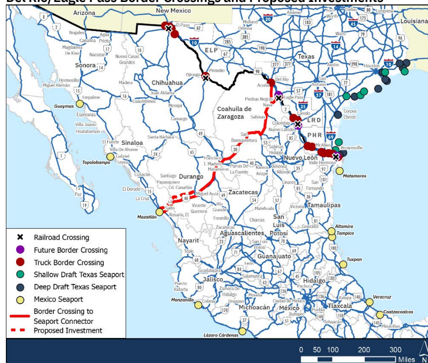
Figure 3-36: Major Corridors Linking Pacific Coast Ports in Mexico to the Del Rio/Eagle Pass Border Crossings and Proposed Investments
