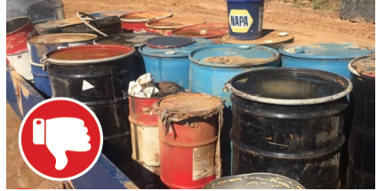
Drums need lids and labels. Storage of hazardous materials should be indoors or in a covered area. Hazardous materials stored onsite should be minimized.
