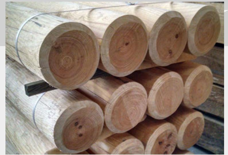
~~Butt slivering due to felling is permitted if the distance from the outside circumference is at least 1/4 of the butt diameter and the height is not more than 1 ft. Use preservative treatment in accordance with AWPA U1, Commodity Specification D.~~ Furnish poles with a minimum net retention of preservative treatment in accordance with Table 1.
