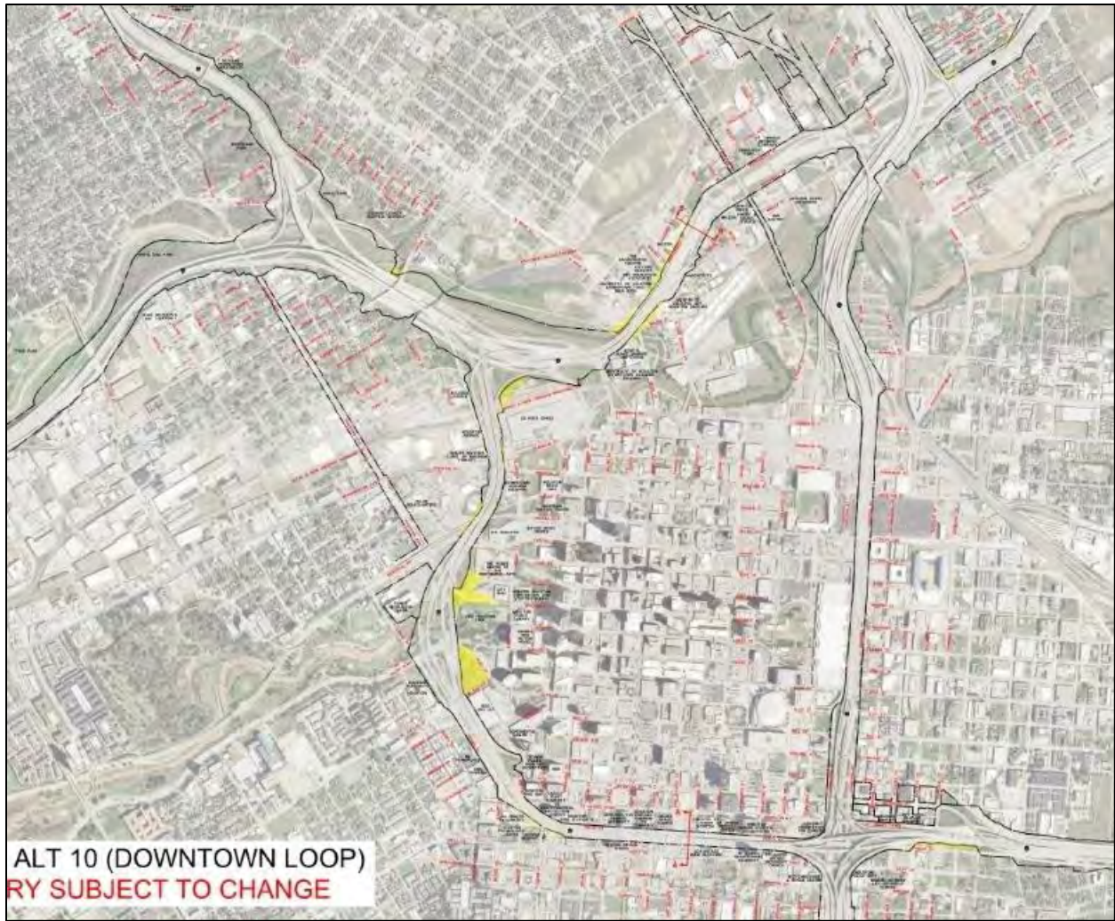
Segment 3/Alternative 10, showing downtown loop area. Proposed ROW acquisition shown in yellow.
