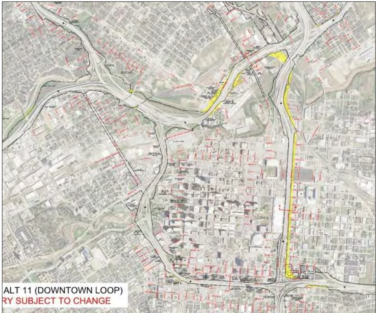
Segment 3/original Alternative 11, showing downtown loop area. Proposed ROW acquisition shown in yellow.
