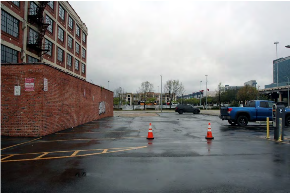
View facing south-southwest. Area of proposed IH 45/IH 69 at center and right of frame. Left orange cone at proposed ROW line, right orange cone at edge of proposed retaining wall for depressed freeway.
