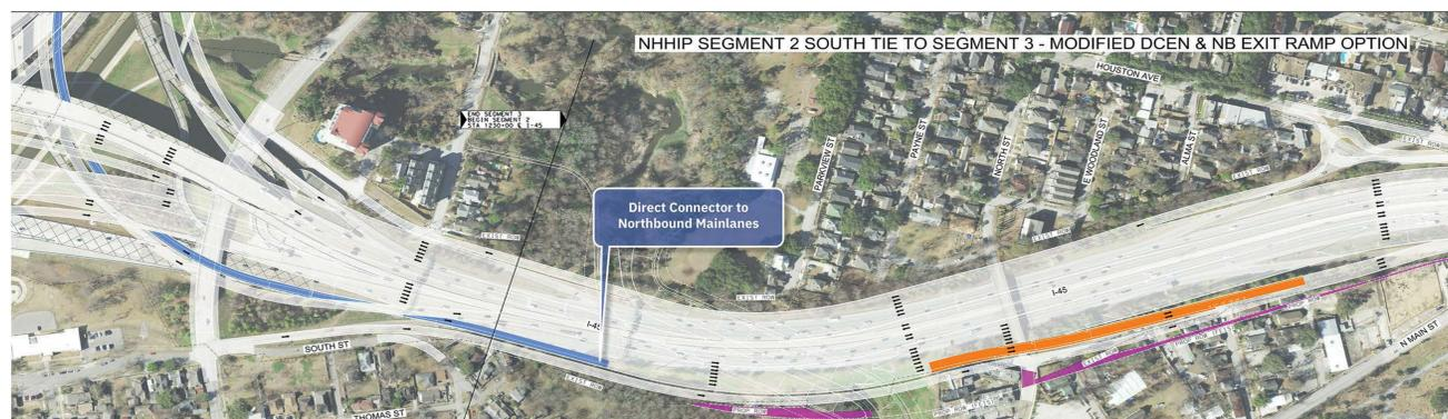
The image above shows in blue the new proposed alignment of the I-10 eastbound direct connector to I-45 northbound. The new configuration allows motorists to enter the I-45 northbound mainlanes instead of going out to the frontage road as before. Not as much space is needed, and the saved ROW is shown in magenta.
