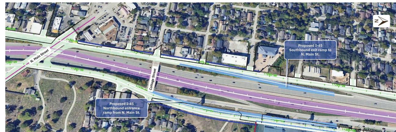
The City of Houston requested that TxDOT include an I-45 southbound exit ramp to N. Main St., as shown in light blue at the top of the image above. Additionally, a design change is being considered to provide an I-45 northbound entrance ramp from N. Main St., indicated in light blue at the bottom of the image. To accommodate this proposed change, Cottage Street may need to be closed for safety reasons due to its close proximity to N. Main St.
