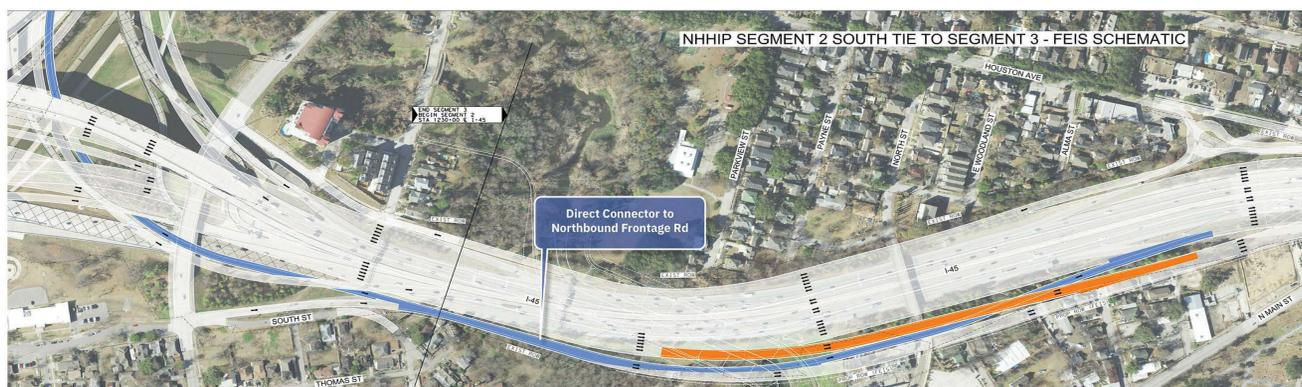
The image above highlights in blue the original alignment of the I-10 eastbound direct connector to I-45 northbound, as approved in the Record of Decision (ROD). This alignment directed motorists out to the I-45 northbound frontage road before they could enter the mainlanes, making additional ROW needed.
