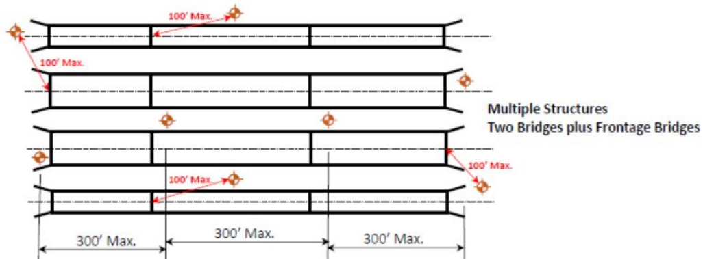
Figure 2-1. Minimum number of test holes for common types of structures
