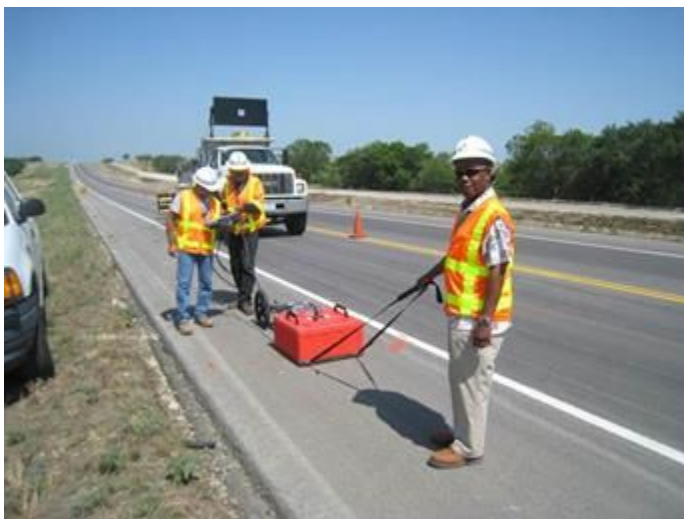
Figure 4-10. 200 MHz Ground-coupled Penetrating Radar.
