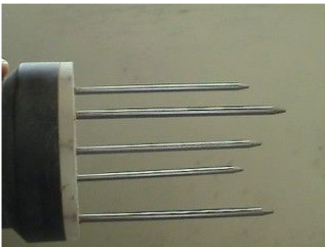
Figure 9-3. Moisture probe for aggregates.
