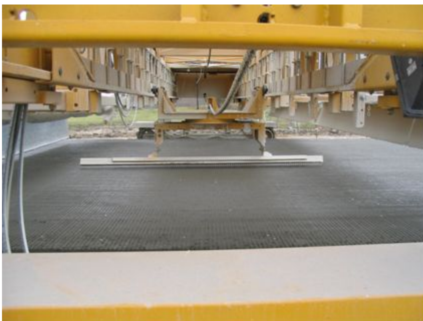
Figure 9-62. Mechanical tining device.
