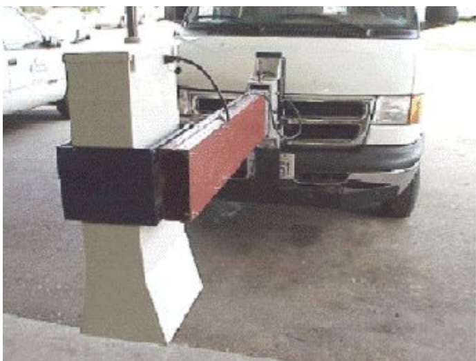
Figure 4-8. Air-coupled Ground Penetrating Radar (GPR).
