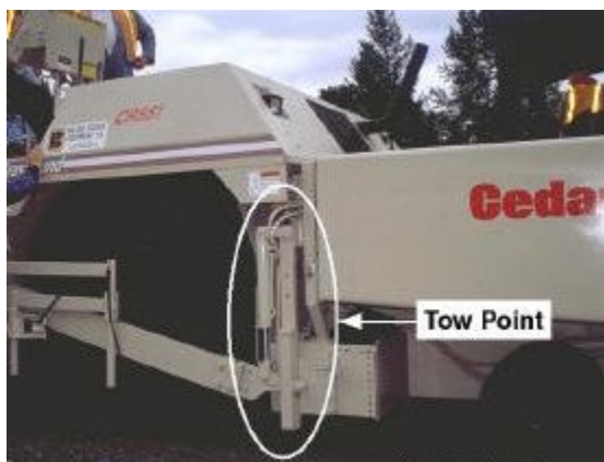
Figure 6-35. Tow Point. © Copyright 2006 University of Washington
