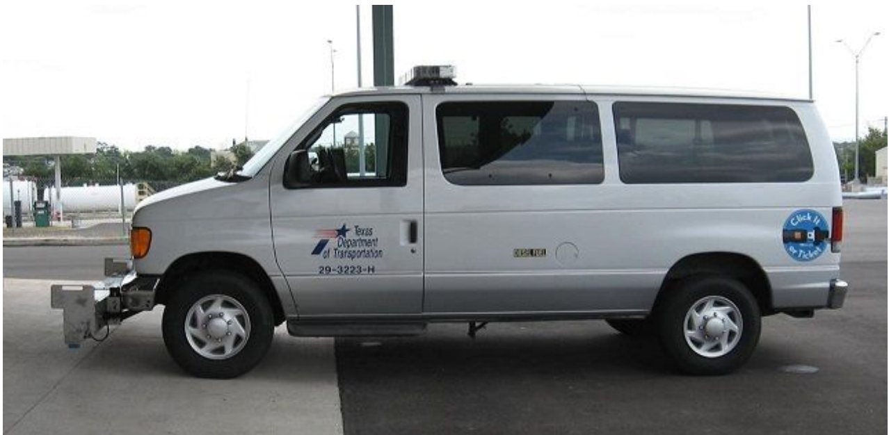
Figure 11-2. High-speed Inertial Profiler with Rut Bar Setup.
