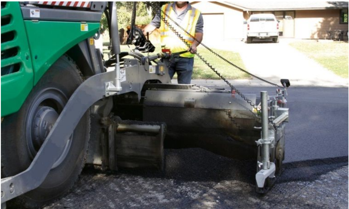
Figure 6-36. Hydraulic Screed Extension. © Copyright 2006 University of Washington
