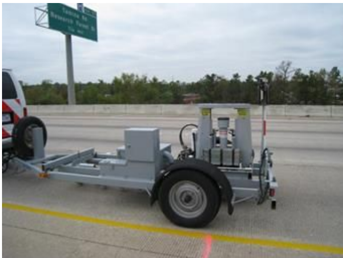
Figure 4-4. Falling Weight Deflectometer (FWD).
