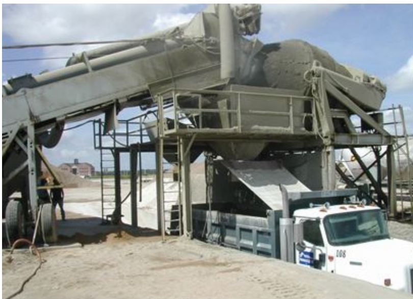
Figure 9-7. Tilting drum mixer.
