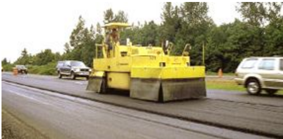
Figure 6-59. Pneumatic Tire Roller (notice rubber skirt insulation around tire area as well as tire marks left in the new mat in front of the roller). © Copyright 2006 University of Washington
