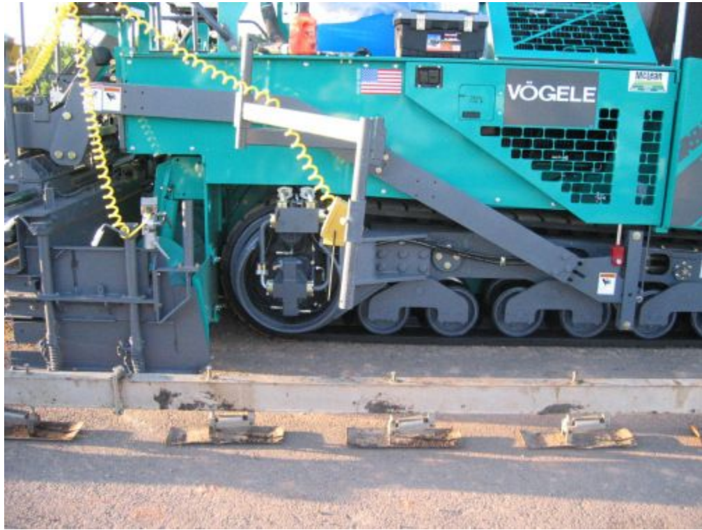
Figure 6-40. Automatic grade control using a mobile reference beam. © Copyright 2006 University of Washington
