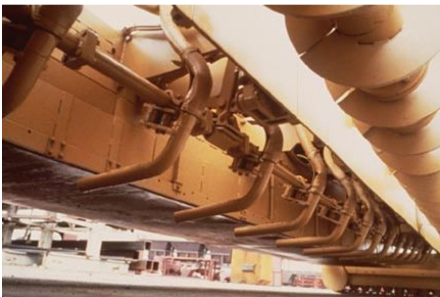
Figure 9-45. Underside of slip-form paver.
