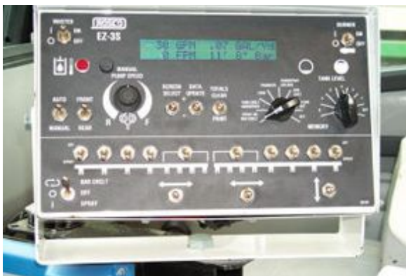
Figure 6-7. Tack Coat Distributor Control Panel. © Copyright 2006 University of Washington
