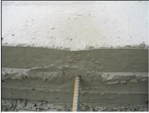
Figure 9-77. Surface drop down due to hand insertion.
