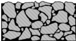
Fig. 3.5a Gap-graded (Performance-Designed or SMA) mix
