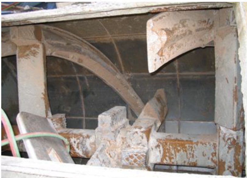
Figure 9-6. Paddles are shown inside a central mix drum.
