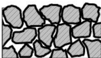
Fig. 3.4a Open-graded (Permeable Friction Course) mix cross section.
