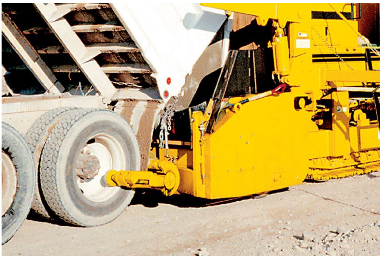
Figure 6-24. Truck hitch engaged. © Copyright 2006 University of Washington
