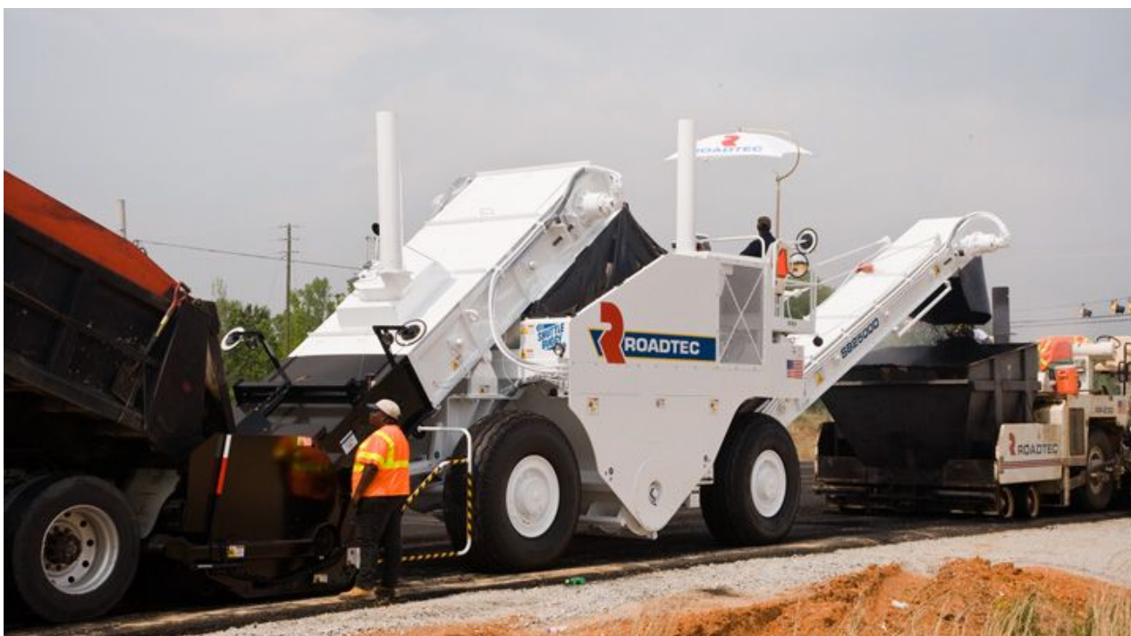
Figure 6-22. Material Transfer Vehicle with surge capacity (Courtesy Roadtec).
