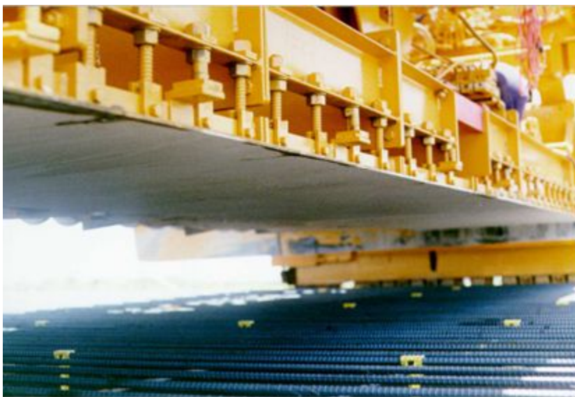
Figure 9-49. Looking up at a pan float on an idle paver.
