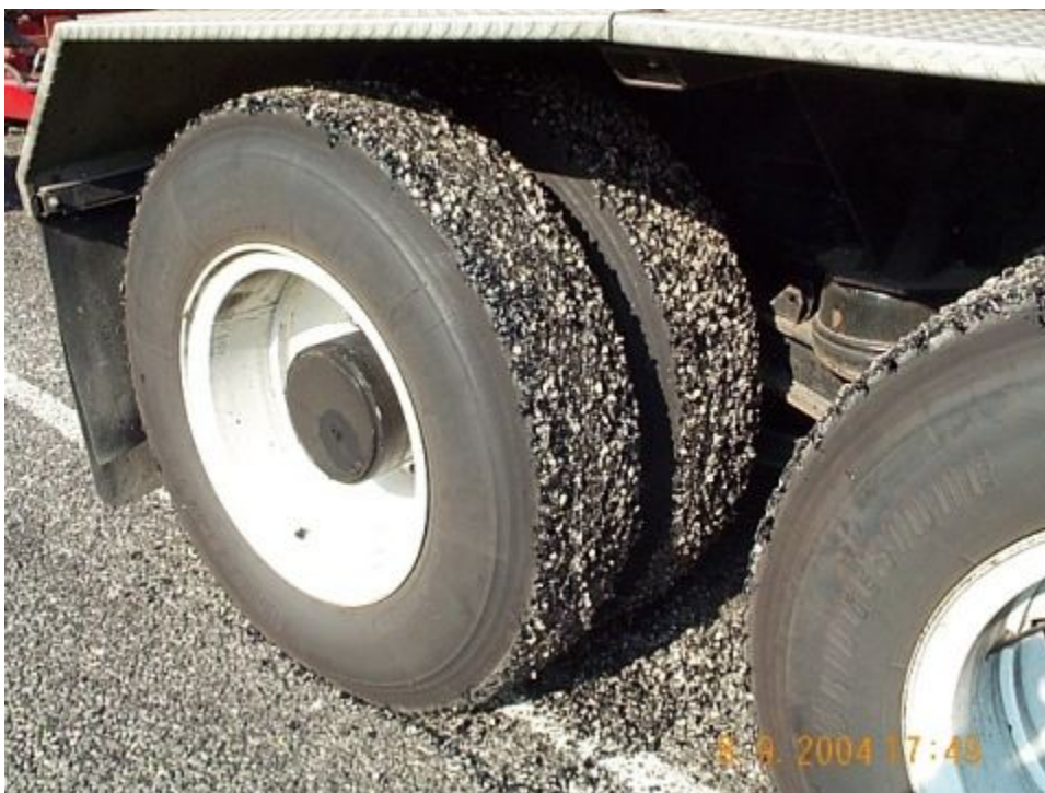
Figure 13-6. Peeling of fresh seal coats (1st photo).
