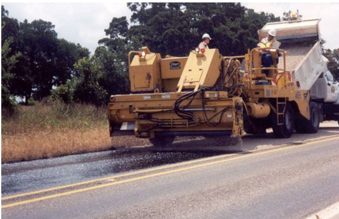
Figure 7-27. Aggregate Spreader or Spreader Box.
