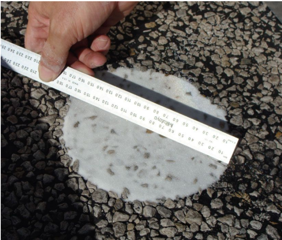
Figure 4-11. Measuring four diameters of the resulting circle for averaging.◆
