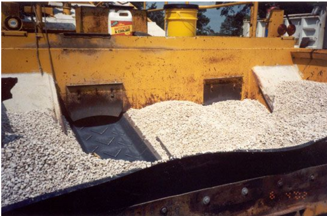
Figure 7-29. Receiving Hopper of Aggregate Spreader.
