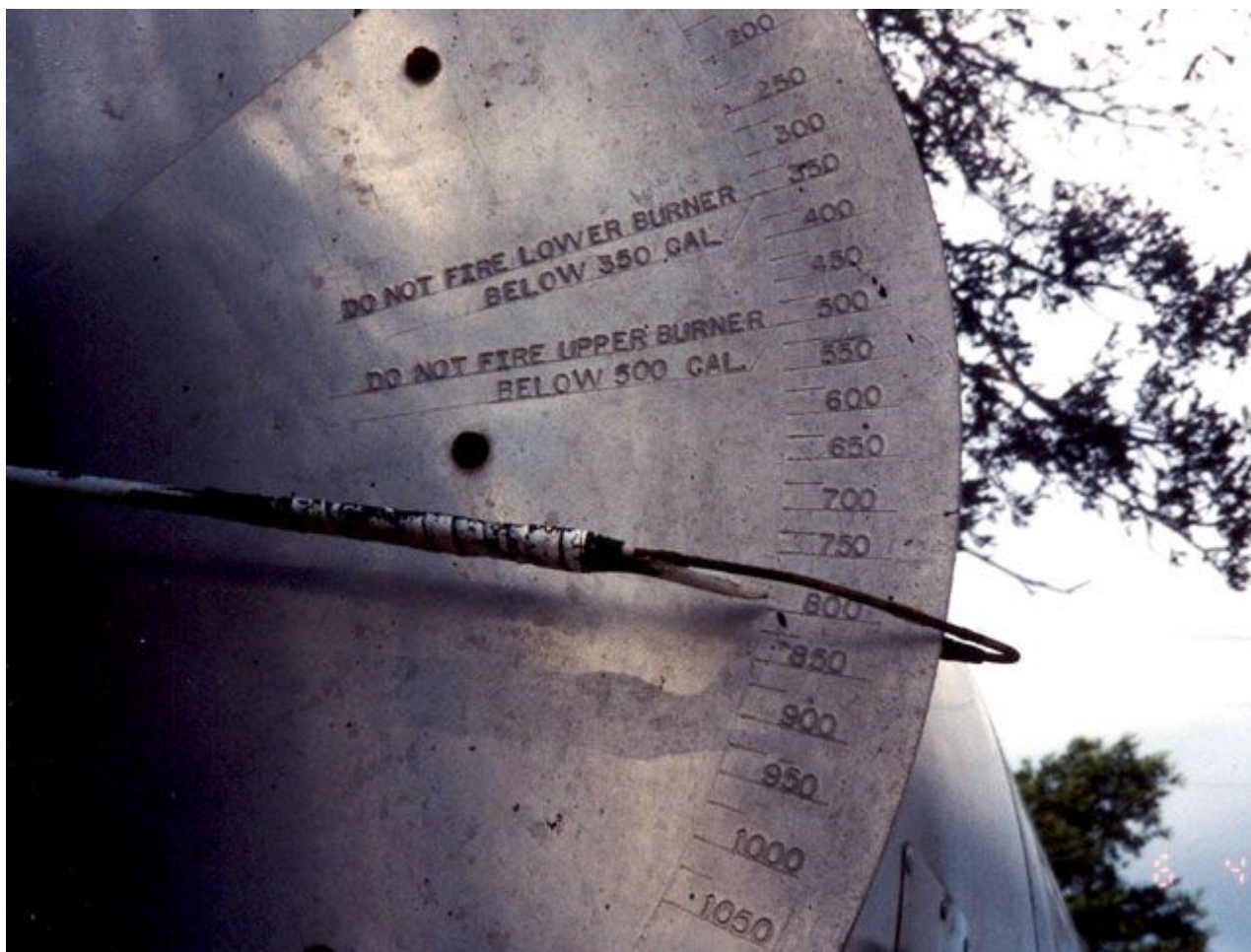
Figure 7-24. Volume Gauge on Distributor Tank.
