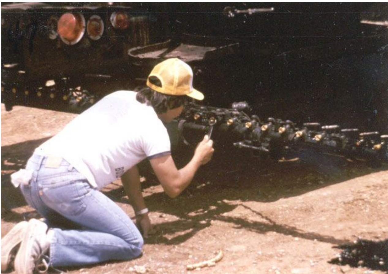
Figure 7-16. Distributor Spray Bar Rotated Outward.
