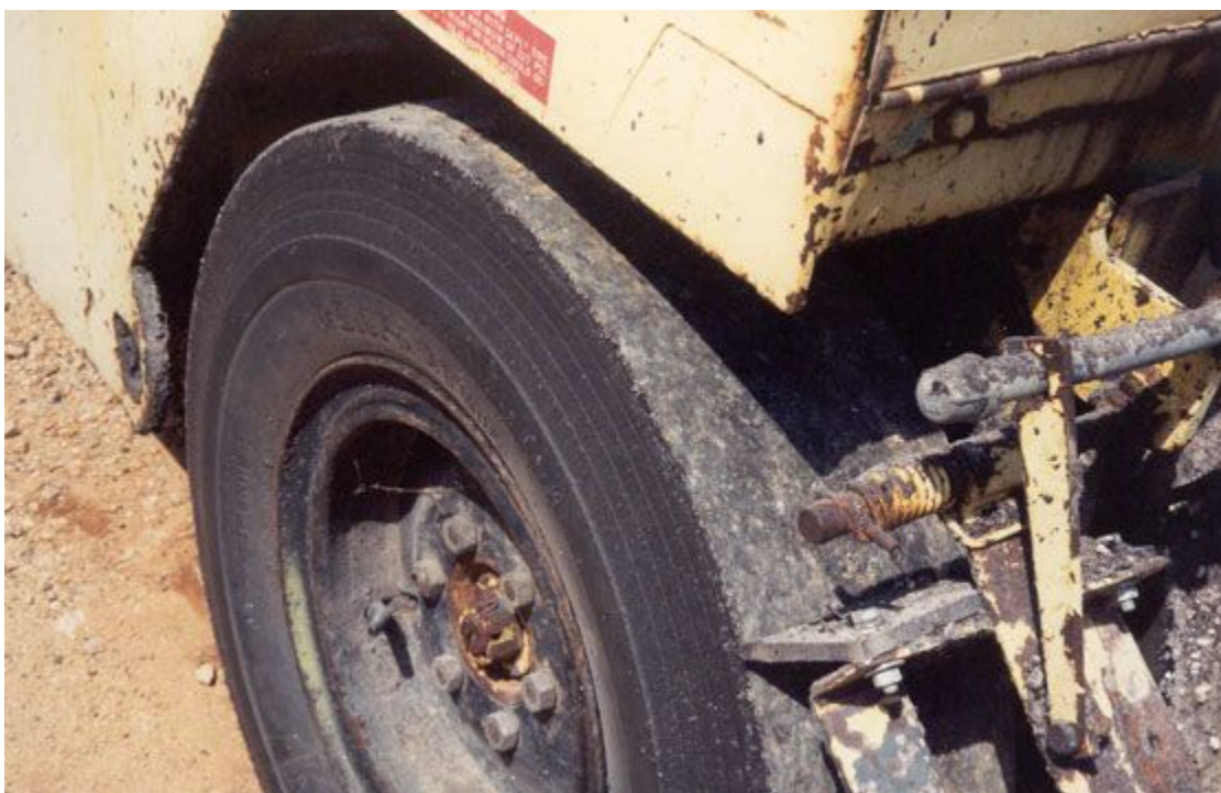
Figure 7-45. Smooth-Surfaced Pneumatic Tire.
