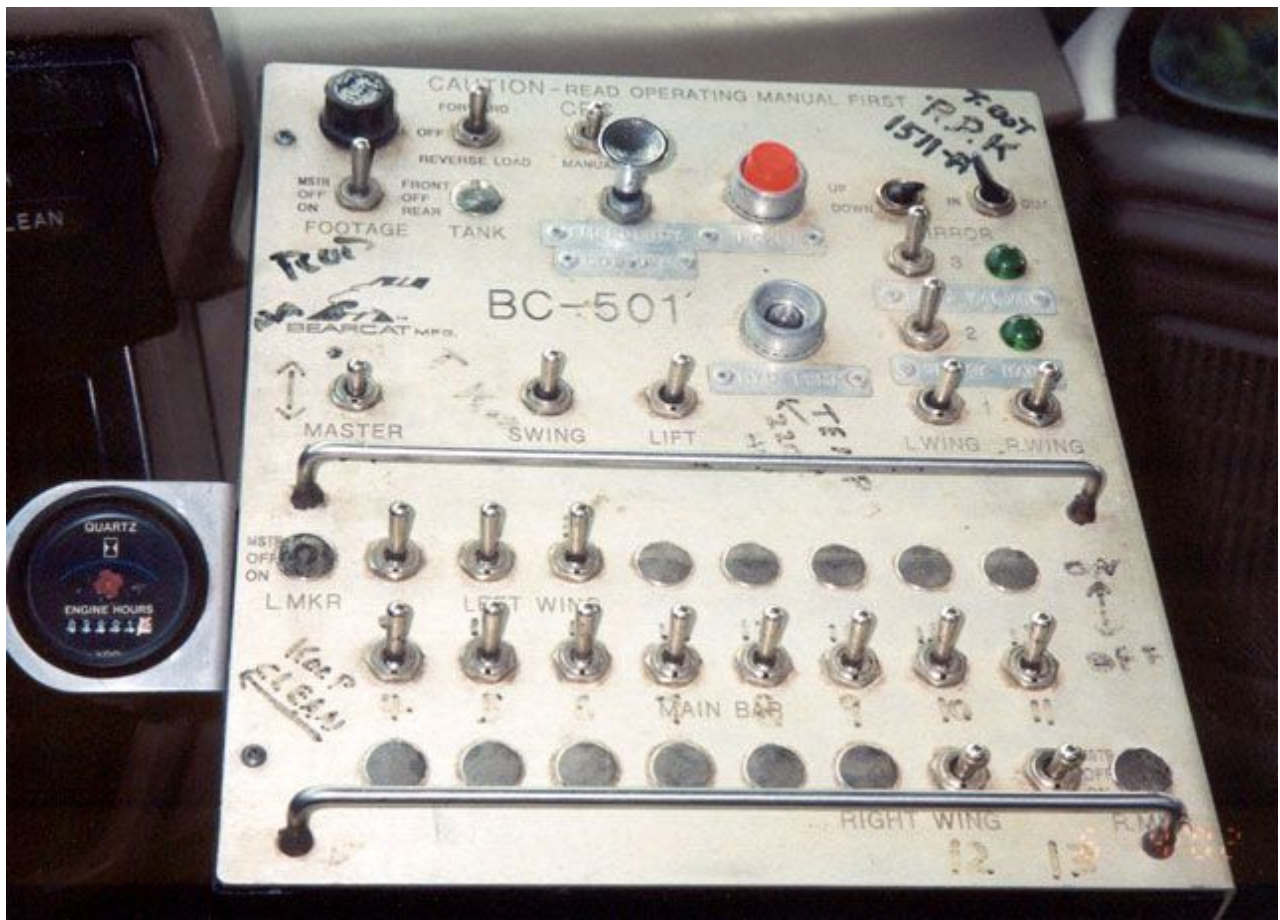
Figure 7-26. Computerized Asphalt Distributor Controls.
