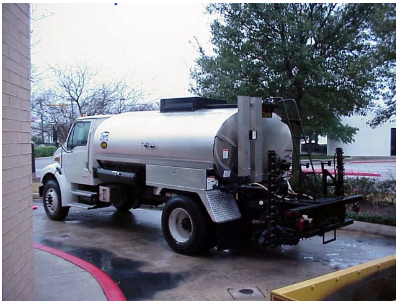
Figure 7-9. Truck-Mounted Asphalt Distributor.
