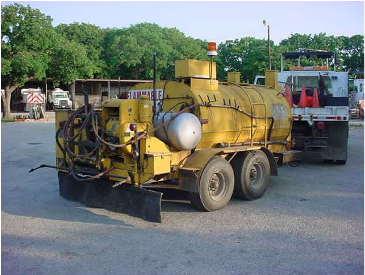
Figure 7-10. Trailer-Mounted Asphalt Distributor.
