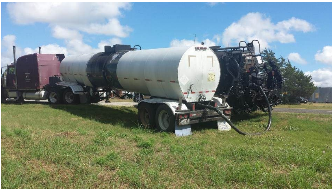
Figure 8-5. Transferring Asphalt from Transporter to Distributor.
