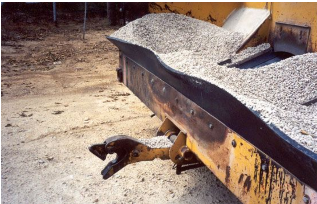
Figure 7-28. Aggregate Spreader Truck Hitch.
