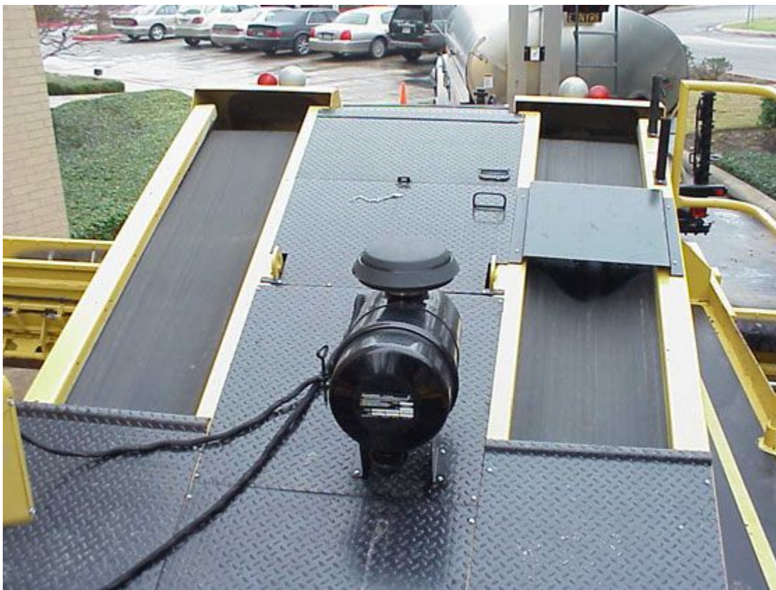
Figure 7-30. Belt Conveyors on Aggregate Spreader.
