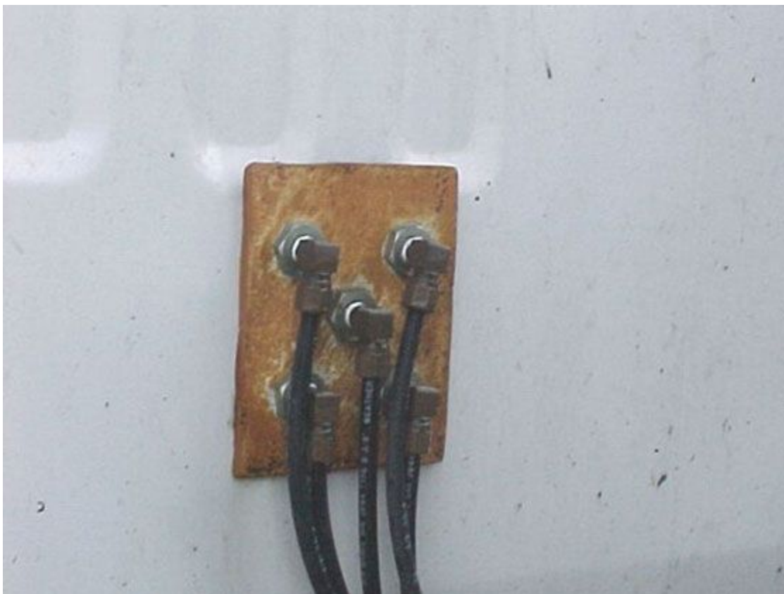
Figure 7-34. Air Line Connections on Back of Truck Cab
