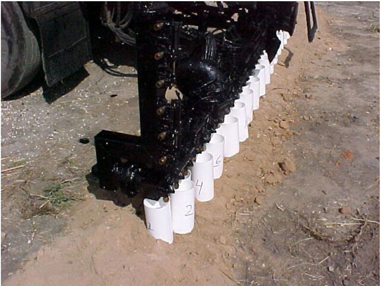
Figure 7-21. Calibration of Asphalt Distributor Spray Bar.
