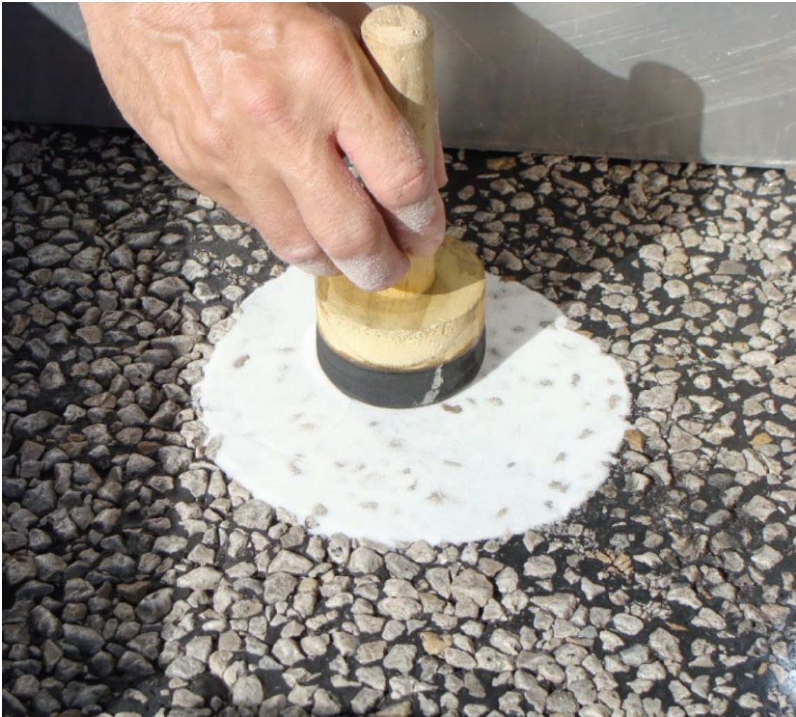
Figure 4-10. Spreading the sand to the level of the highest aggregates. ♦
