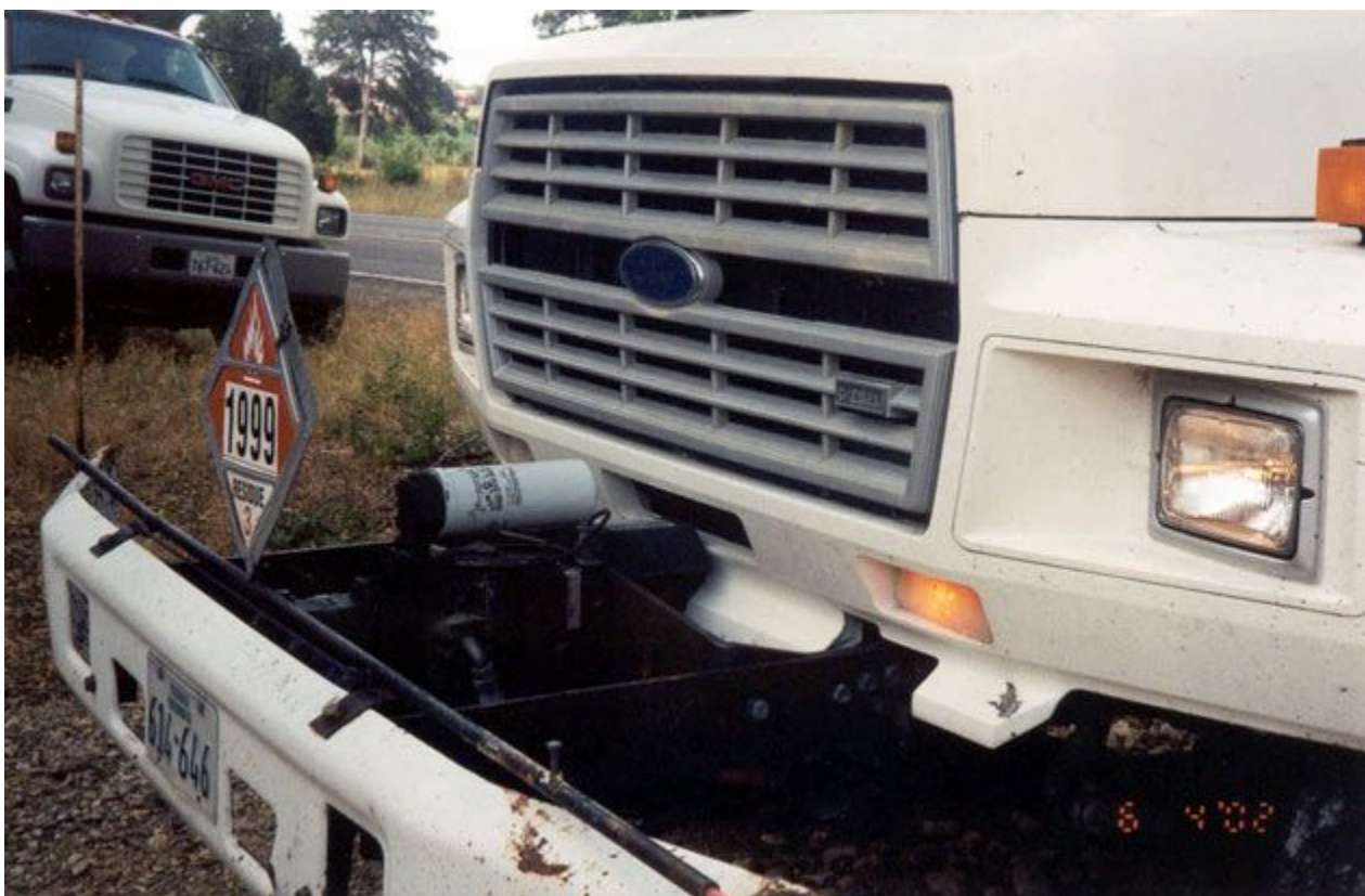
Figure 7-8. Hydrostatic Distributor Located at Front of Truck.
