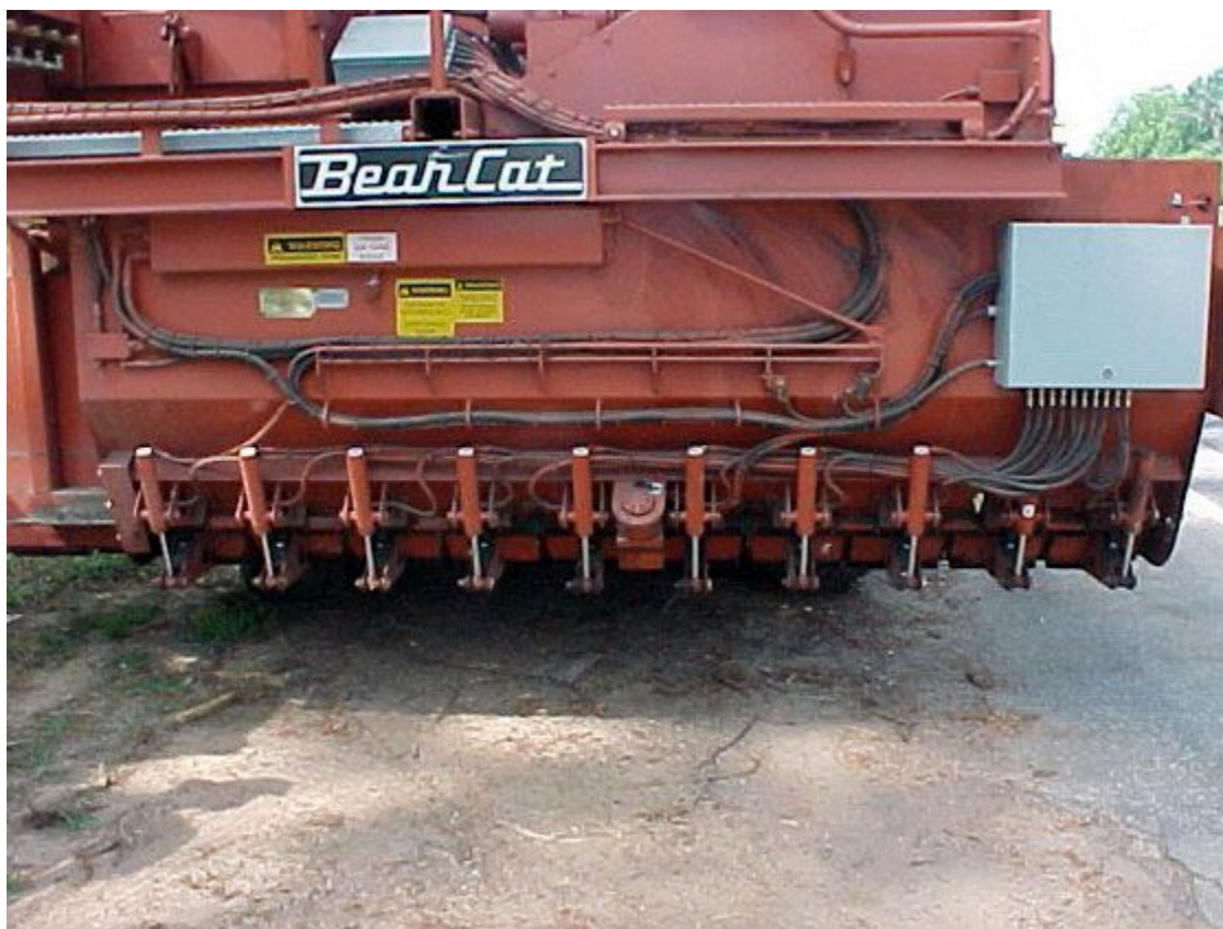
Figure 7-32. Discharge Gates on Aggregate Spreader.
