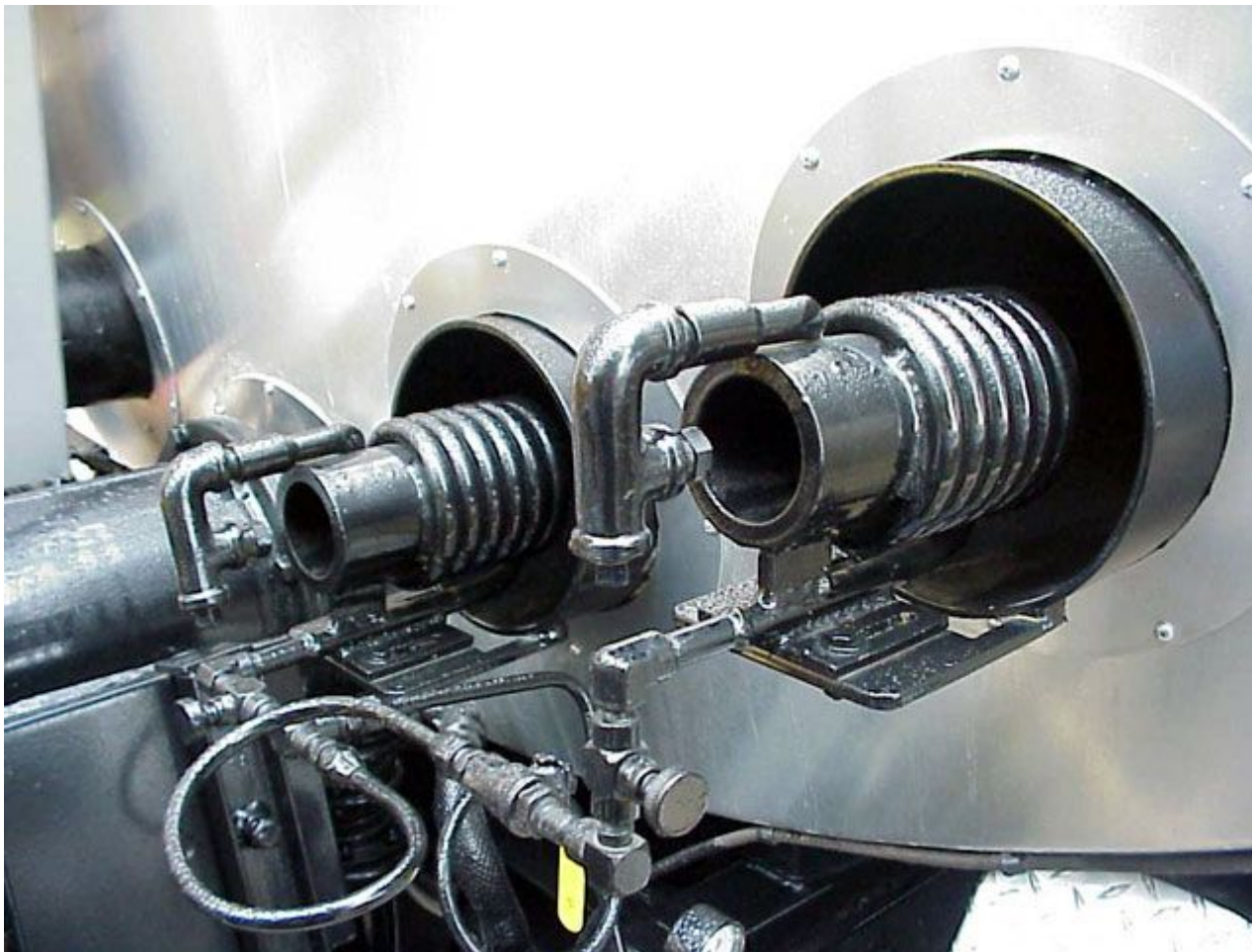
Figure 7-7. Burner Configuration at Rear of Tank.
