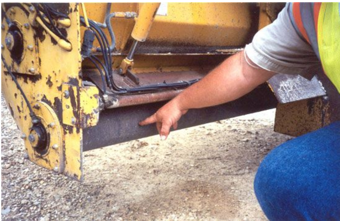
Figure 7-33. Discharge Roller on Aggregate Spreader.
