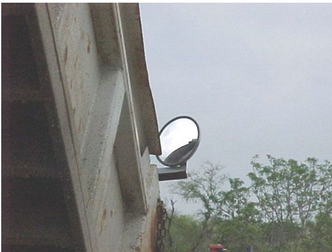
Figure 7-36. Mirror to View Rock in Truck and Rock Flow
