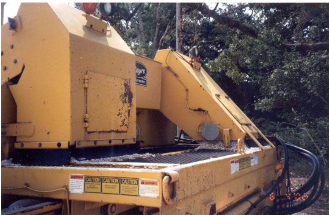
Figure 7-31. Discharge Hopper of Aggregate Spreader.
