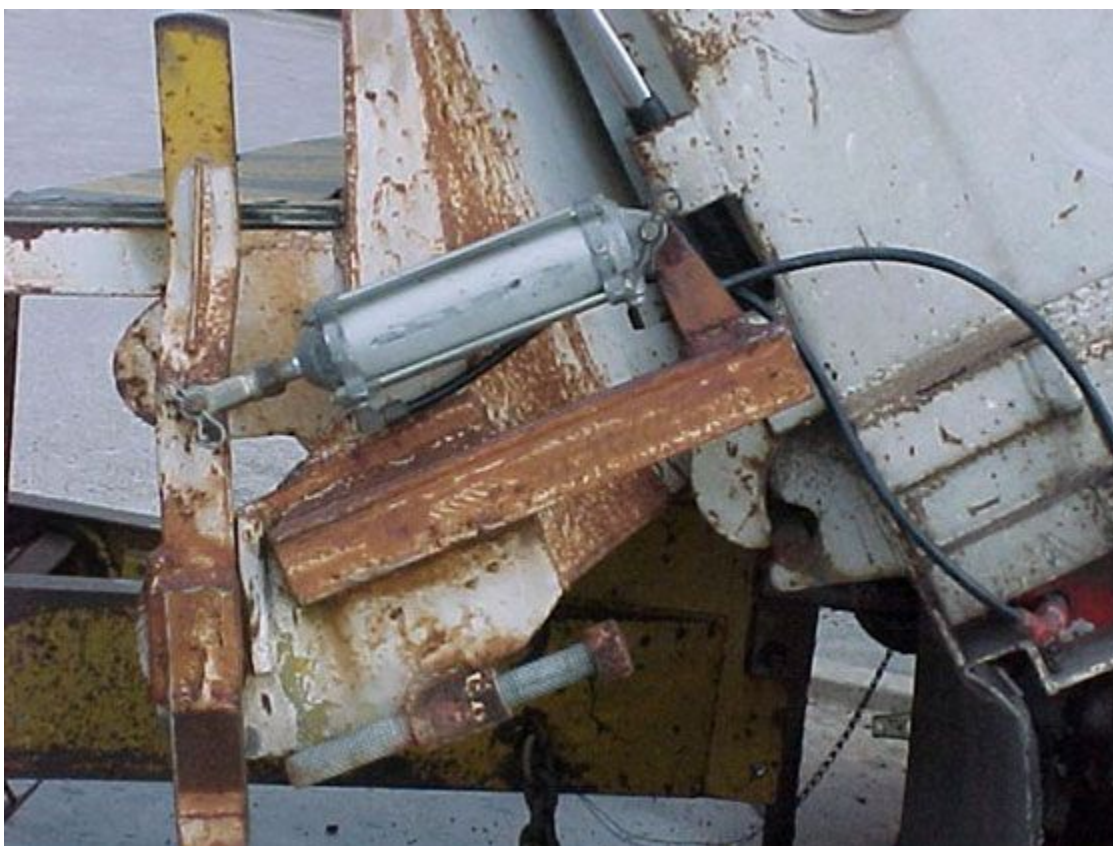
Figure 7-37. Air Cylinder to Open/Close Spreader
