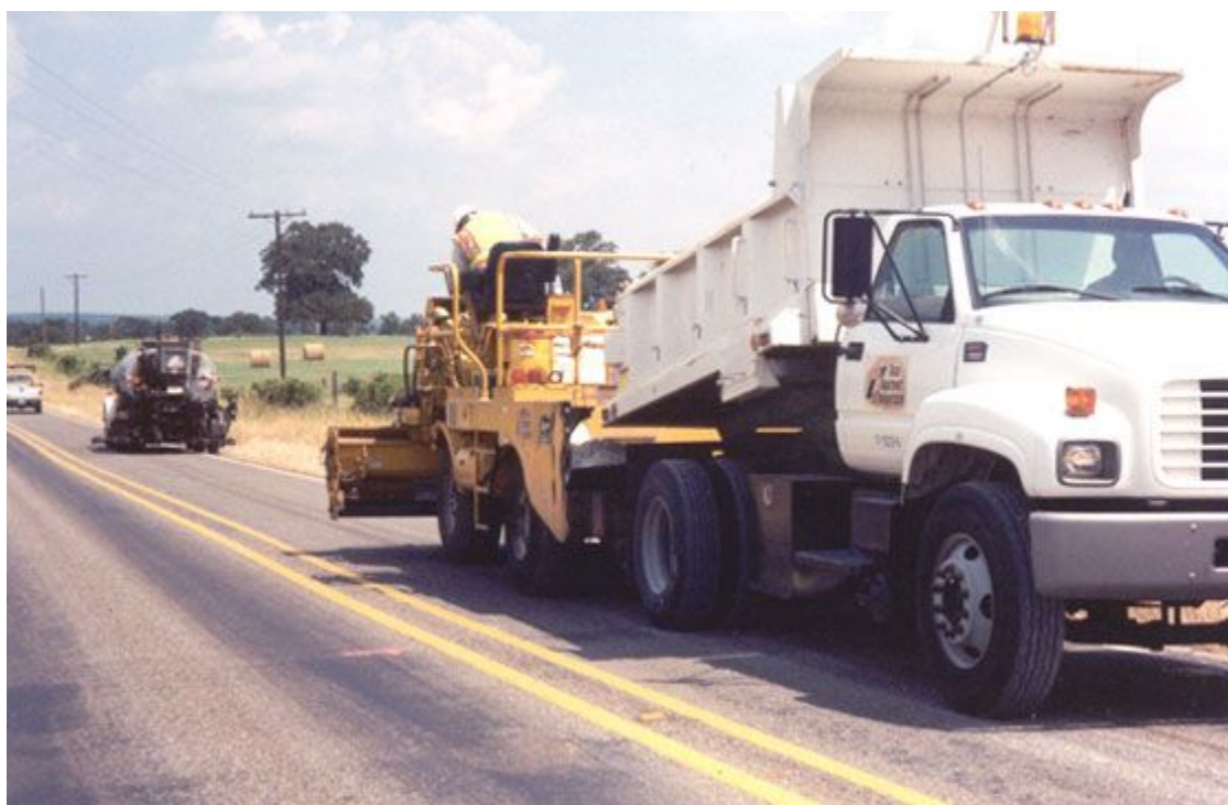
Figure 7-38. End-Dump, Single-Axle Aggregate Haul Truck.
