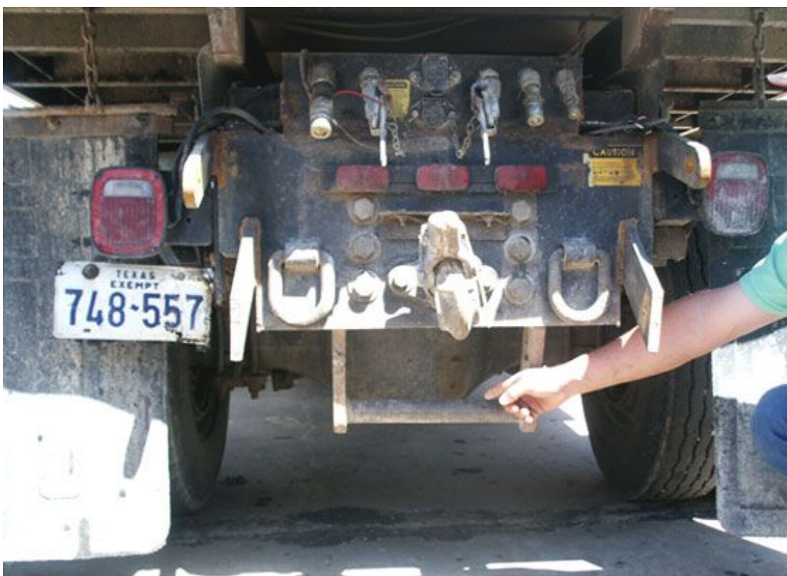
Figure 7-40. Truck Hitch to Connect to Aggregate Spreader.
