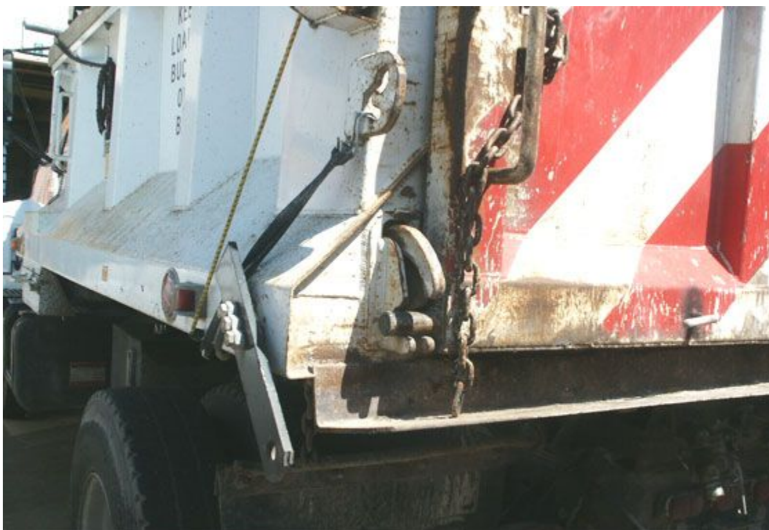
Figure 7-39. Latch on Tailgate of Haul Truck.
