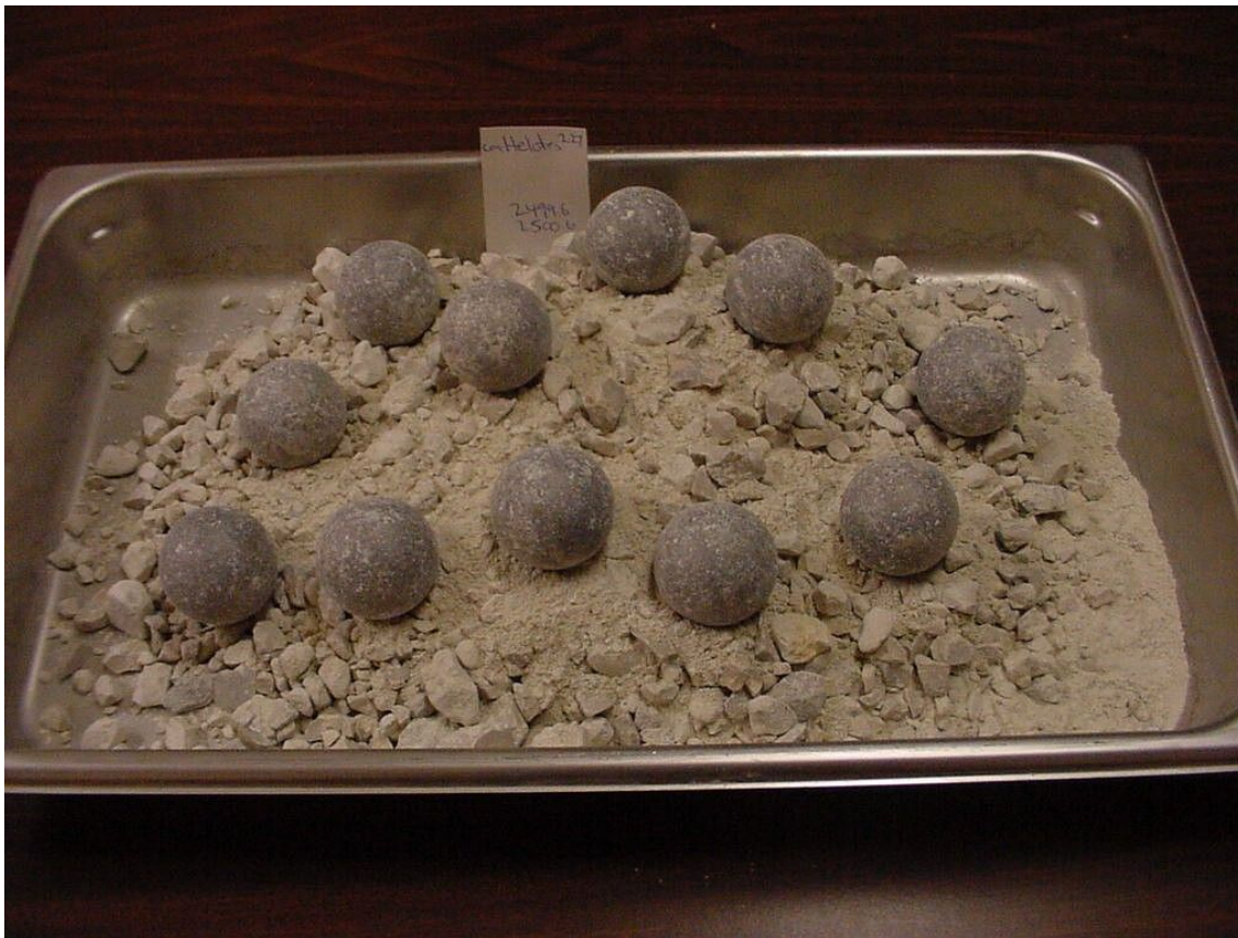
Figure 3-6. Aggregate before and after Los Angeles Abrasion test. ♦
