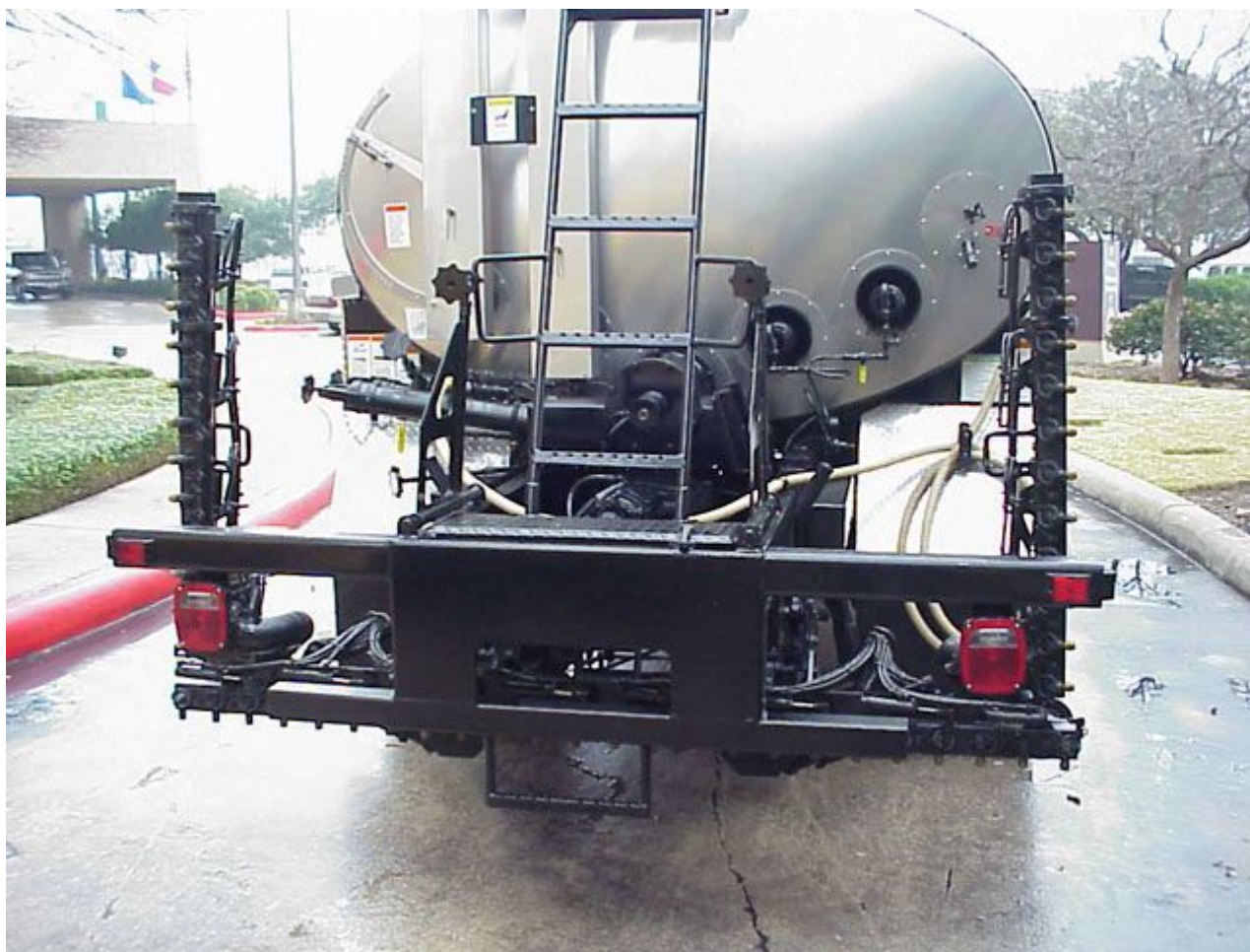
Figure 7-13. Hinged Spray Bar with Ends Folded Up.
