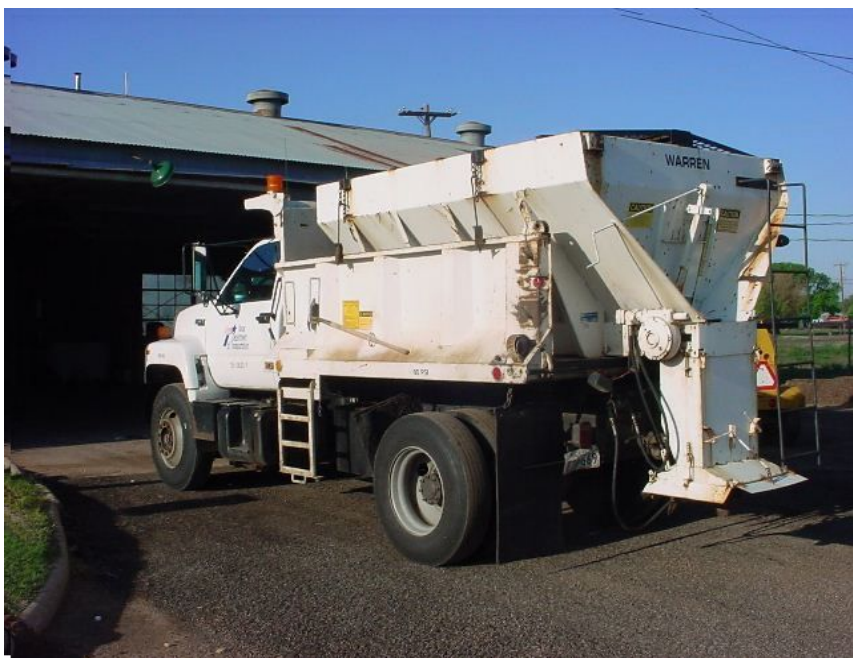
Figure 3-6. Tail gate spreaders are used to apply de-icing and anti-icing materials. They are a spinner type applicator and operate via a hydraulic system.
