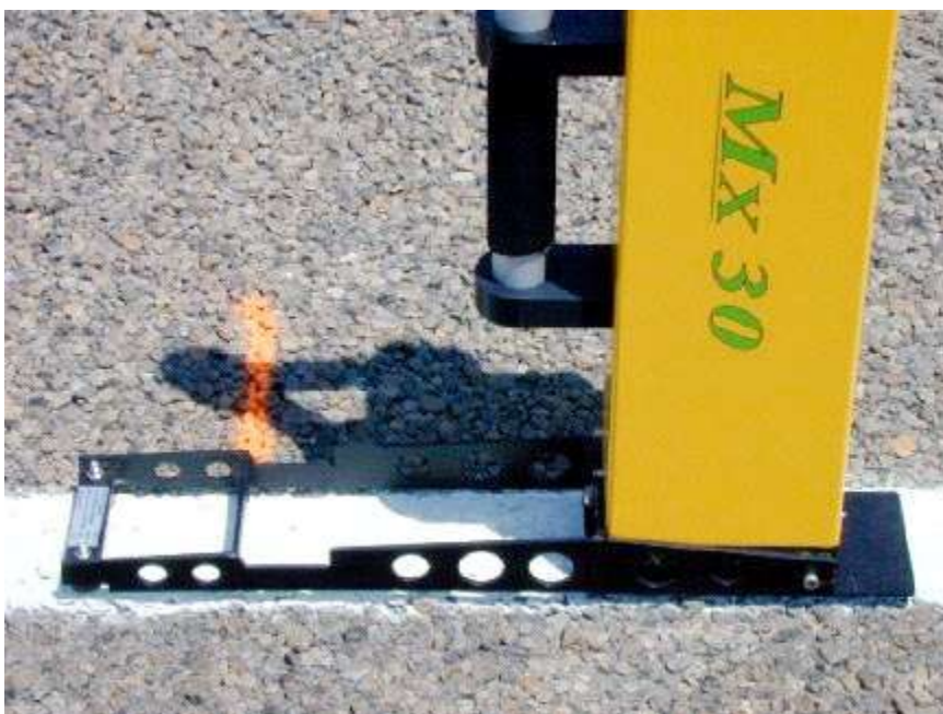
Figure 3-6. Handheld instrument prepared for retroreflectivity measurement.
