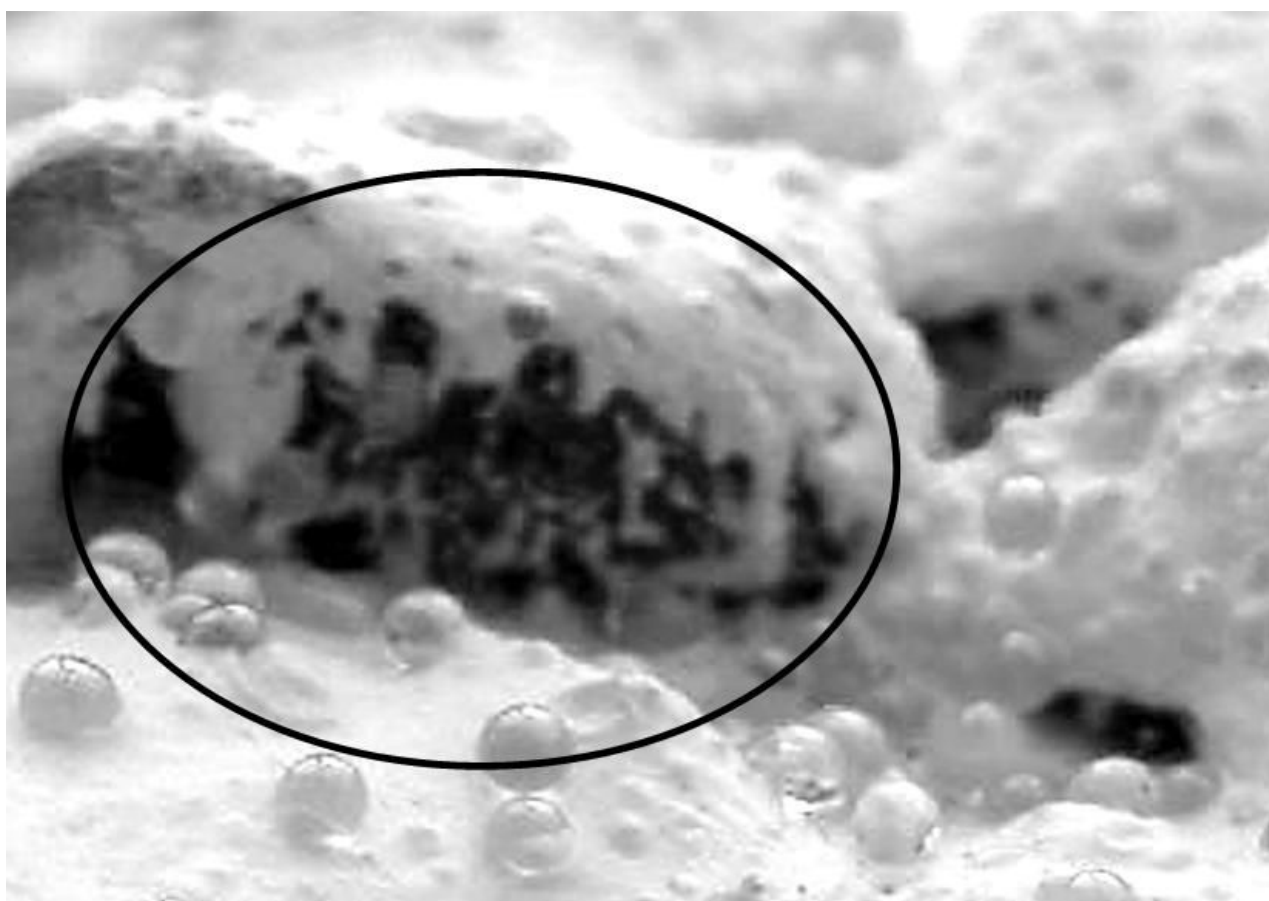
Figure 2-4. Poor material coverage on backside of aggregate.
