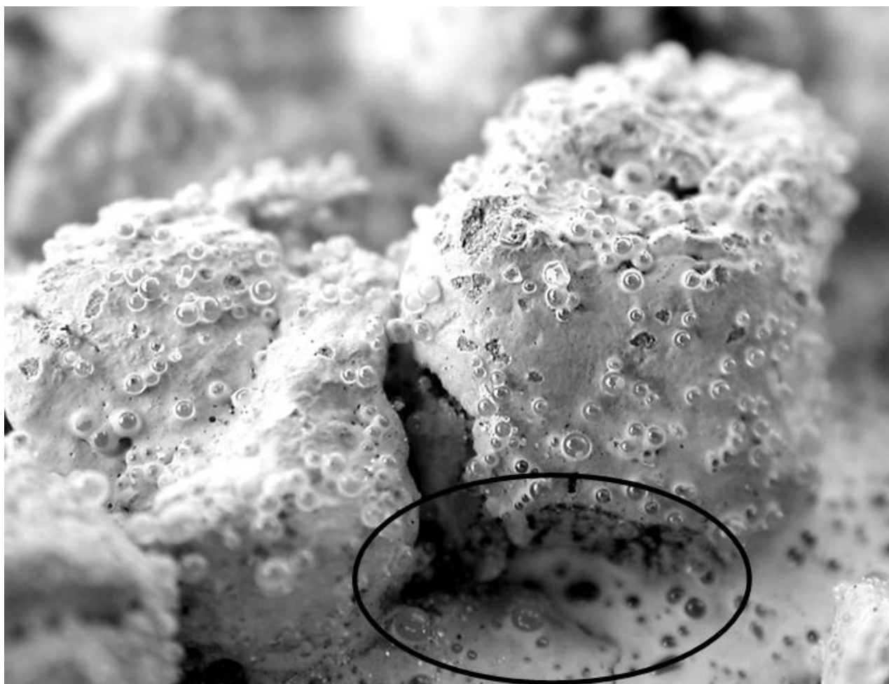
Figure 2-2. Beads falling between aggregates.
