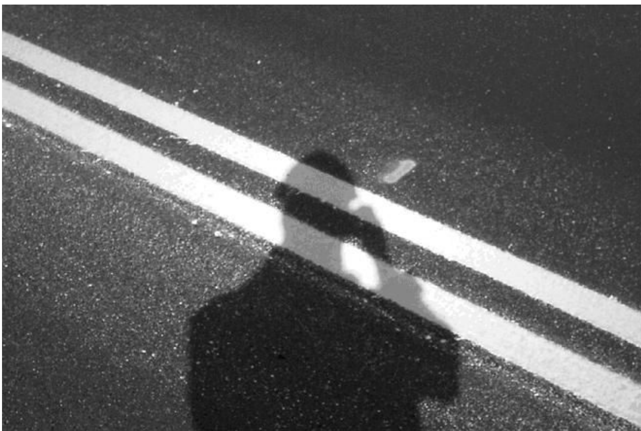
Figure 3-5. Sun-over-shoulder test from Test Method Tex-828-B.
