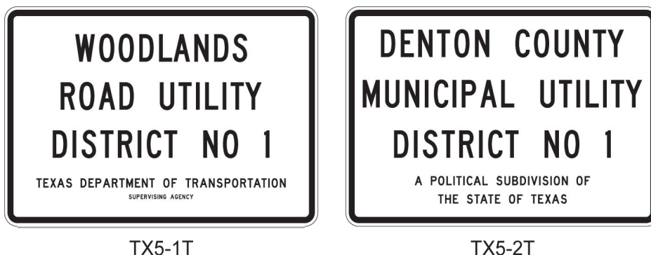
Figure 8-3. Typical utility district signs. Background is white reflective; border and legend are black. The three upper lines are for the district name. Variations in the number of letters per line will depend on the length of the district name.
