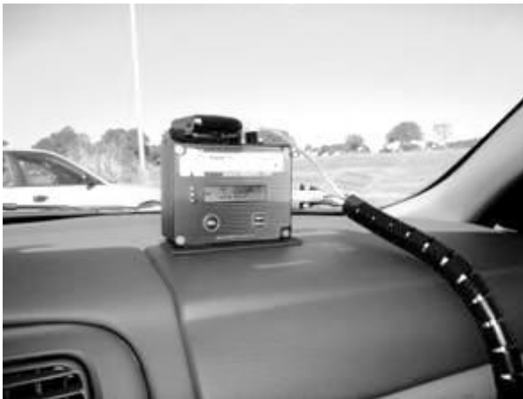
Figure 5-4. Equipment setup in test vehicle-GPS positioning.
